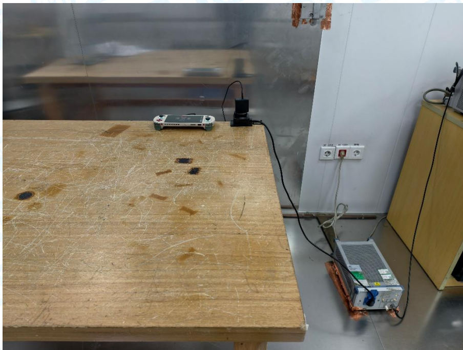
Photo of Setup for Conducted Emission
