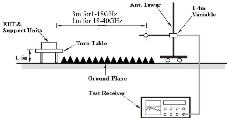
The setup of EUT is according with per ANSI C63.10-2013 measurement procedure. The specification used was with the FCC 15.209 and FCC 15.407 limits.
