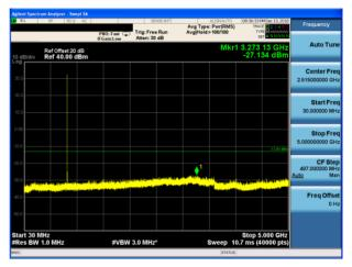
Conducted Emission Transmitting Mode CH 128 5GHz – 10GHz
