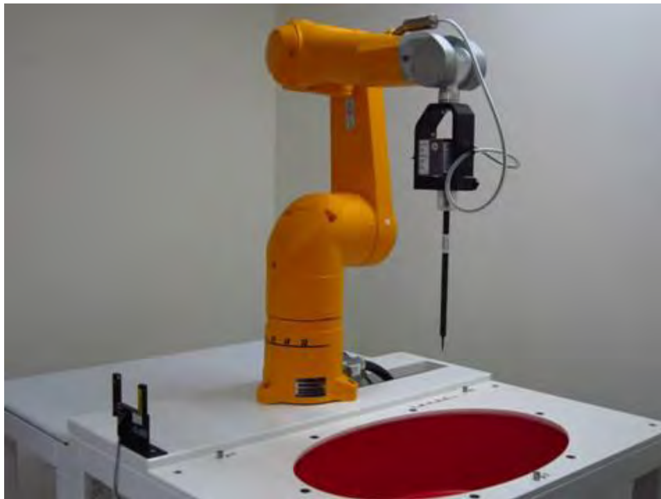
Fig.1 Photograph of the SAR measurement system
