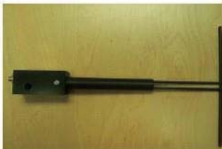
Figure 1 – MVG COMOSAR Validation Dipole
