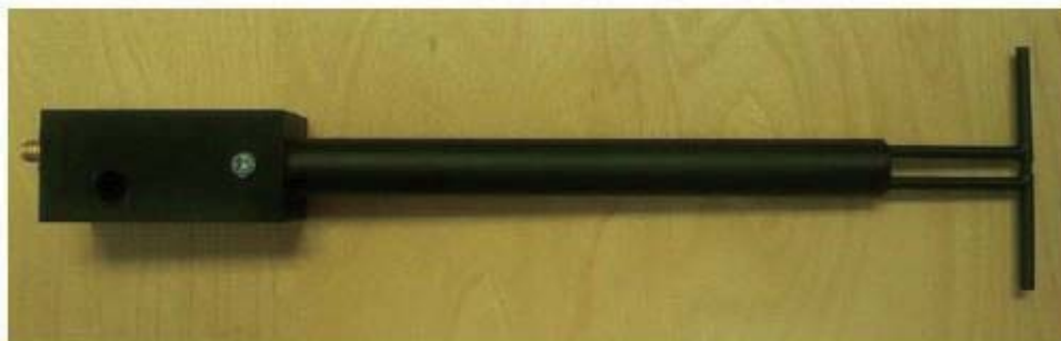
Figure 1 – MVG COMOSAR Validation Dipole
