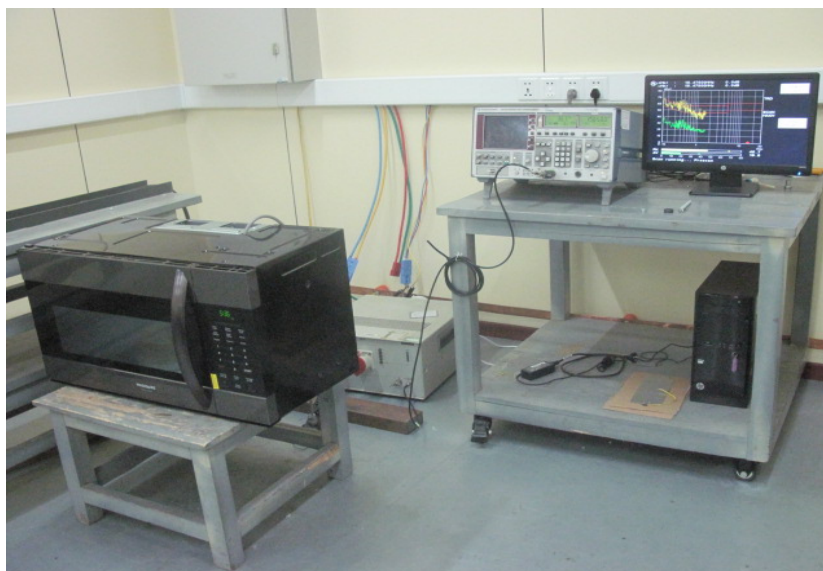
Conducted Emission Test Set-up
