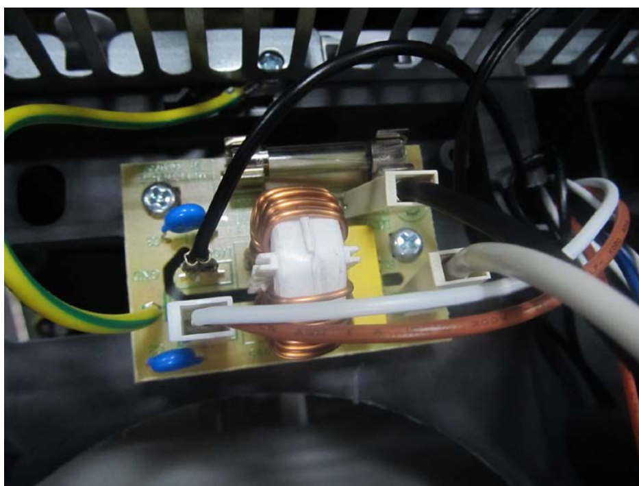
Power Filter Board- Top View
