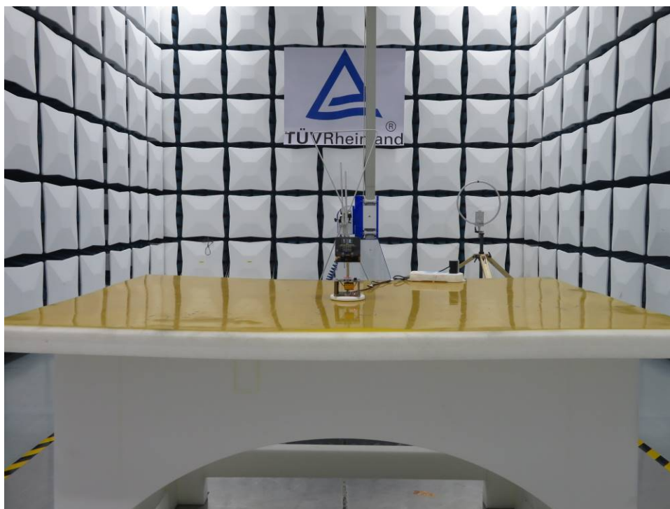
Photograph 2: Set-up photo for Radiated Spurious Emission, 30MHz - 1GHz
