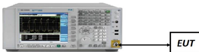
Figure 7-3. Test Instrument & Measurement Setup
