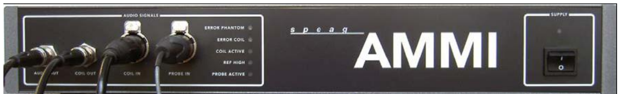
Figure 5.3 AMMI front panel
