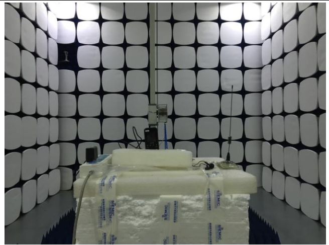
Radiated Spurious Emissions Test Setup Above 1GHz
