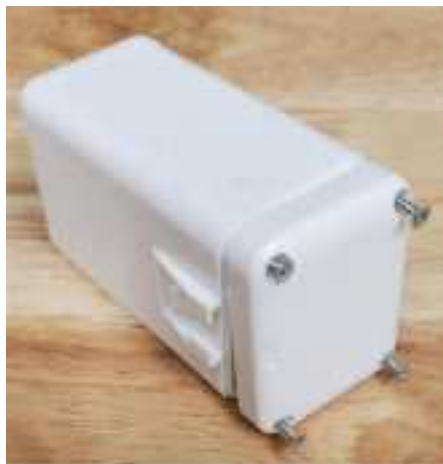
Figure 2-5: Removing the Battery Cover Screws
