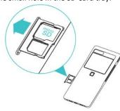
Remove the SD Card tray from the ChecOut M device. When reinserting the SD card, ensure that it is in the proper orientation relative to the tray.
