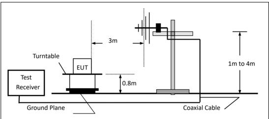
(c) For radiated emissions above 1000MHz
