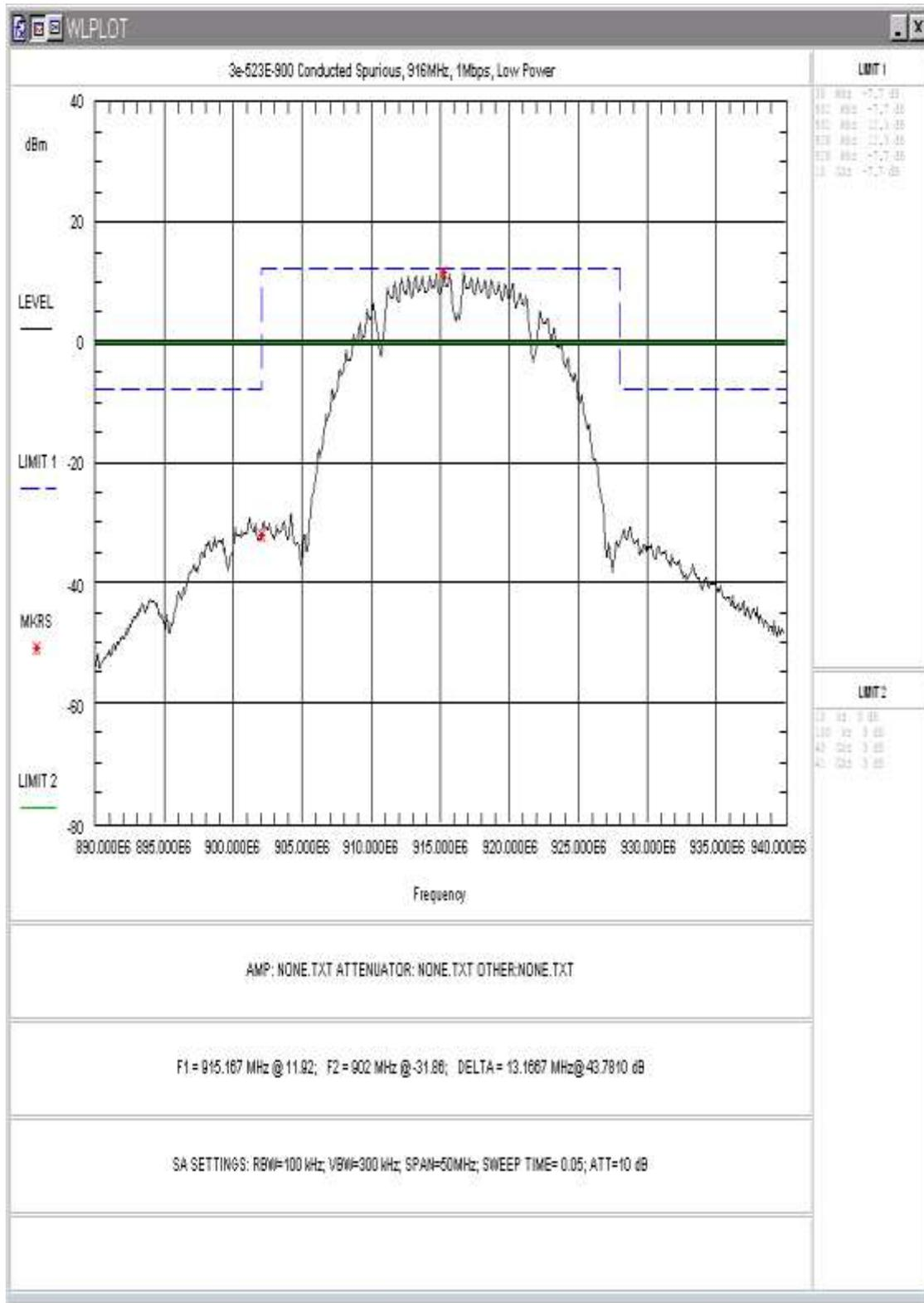
Figure 14: Conducted Spurious Emissions, 1Mbps, Low Power, 890-940MHz
