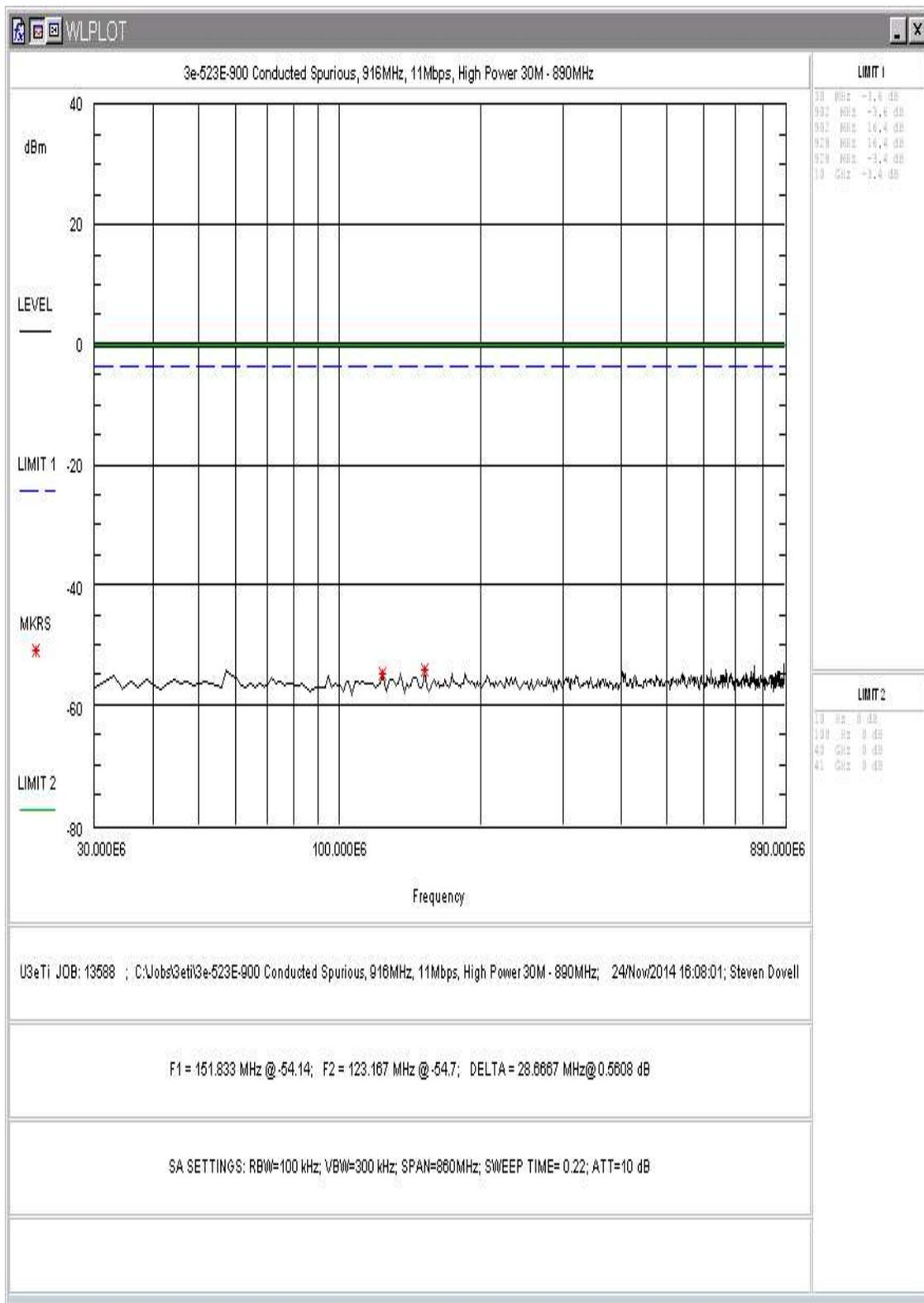
Figure 9: Conducted Spurious Emissions, 11Mbps, High Power, 30 - 890MHz
