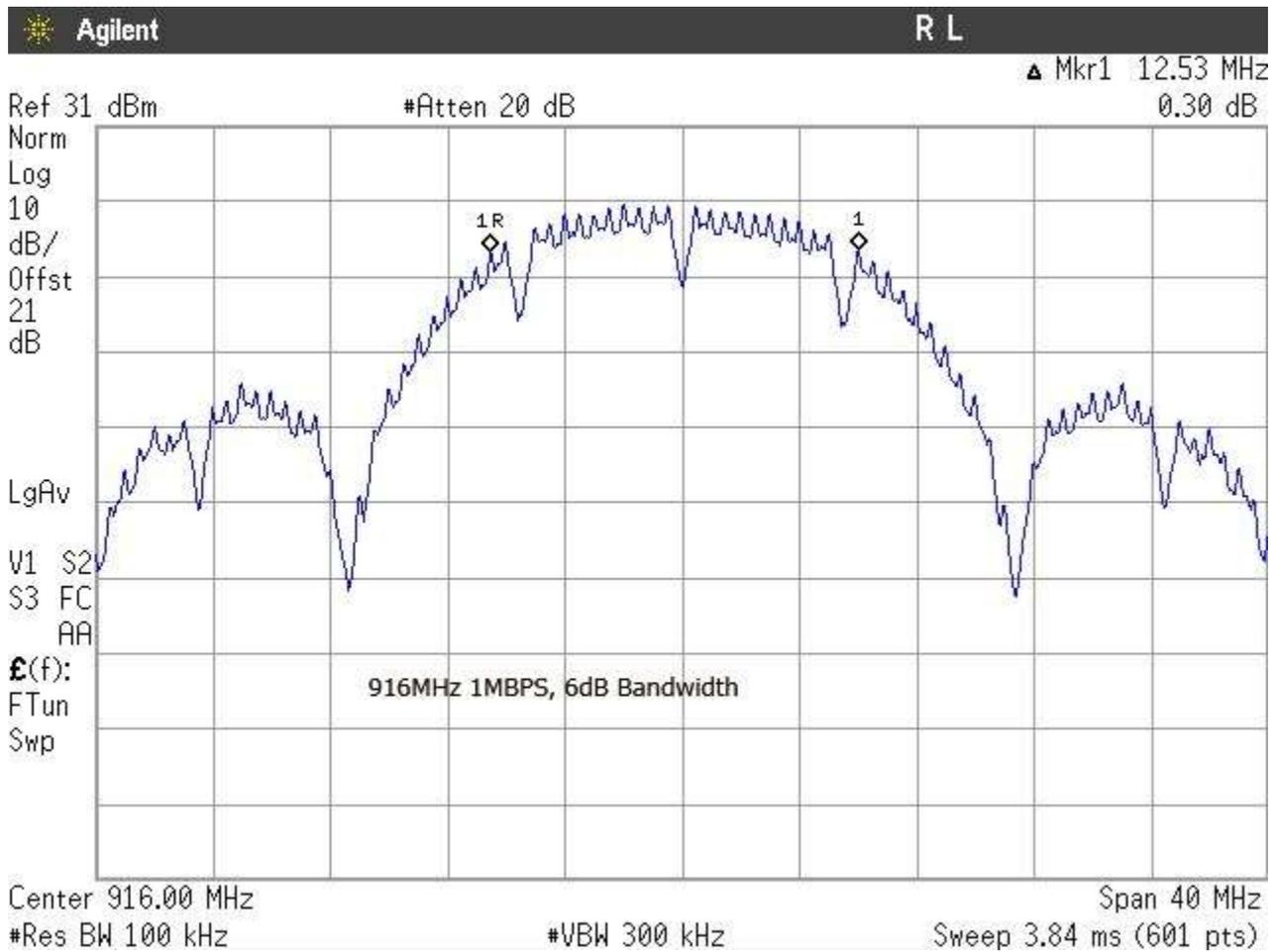
Figure 1: Occupied Bandwidth, 916MHz, 1Mbps
