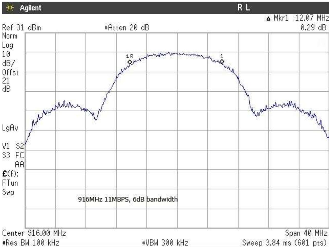
**Figure 2: Occupied Bandwidth, 916MHz, 11Mbps**
