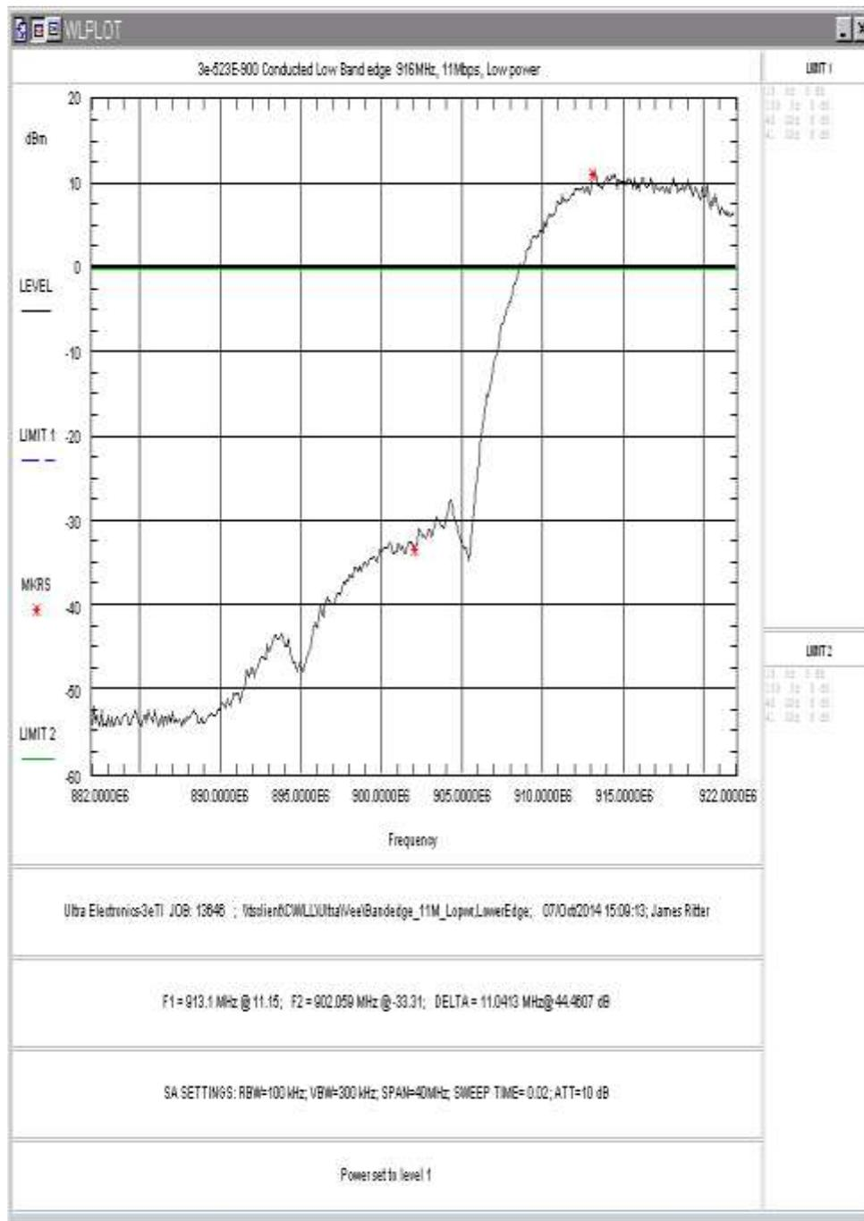
Figure 24: Lower Band-edge, 11Mbps, Low Power
