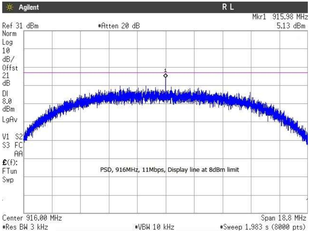
Figure 4: Power Spectral Density, 916MHz, 11Mbps
