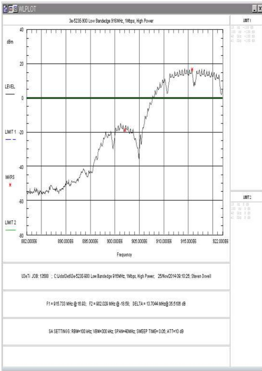
Figure 21: Lower Band-edge, 1Mbps, High Power
