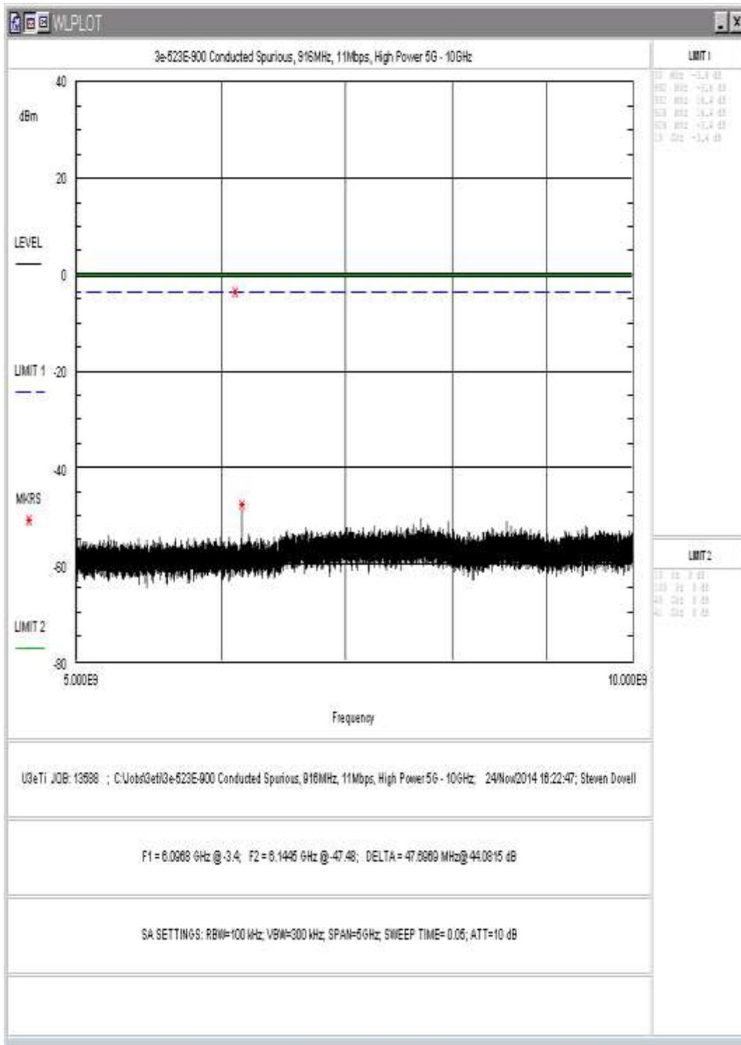
Figure 12: Conducted Spurious Emissions, 11Mbps, High Power, 5-10GHz
