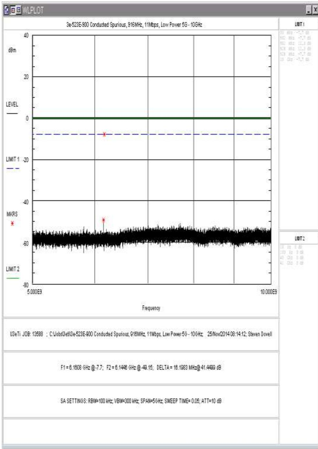
Figure 20: Conducted Spurious Emissions, 11Mbps, Low Power, 5-10GHz
