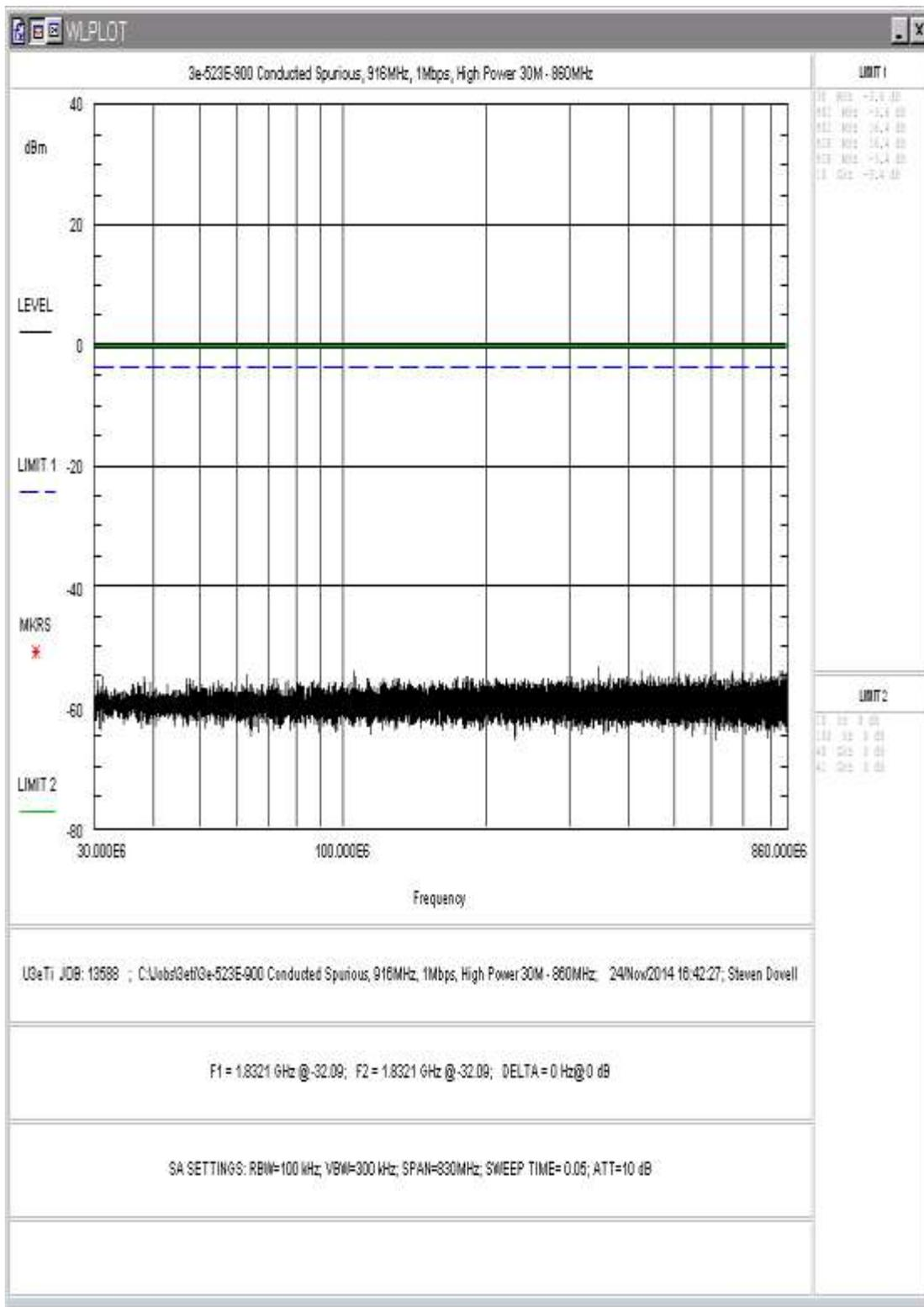
Figure 5: Conducted Spurious Emissions, 1Mbps, High Power, 30 - 890MHz
