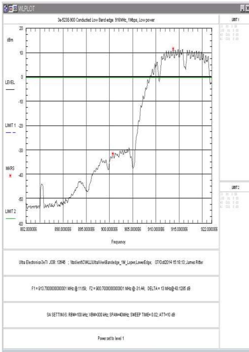
Figure 23: Lower Band-edge, 1Mbps, Low Power
