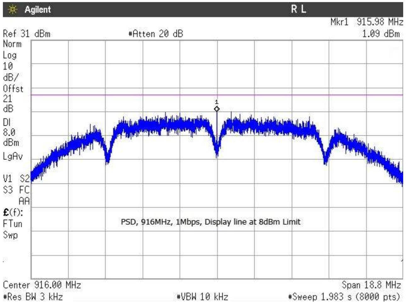
Figure 3: Power Spectral Density, 916MHz, 1Mbps
