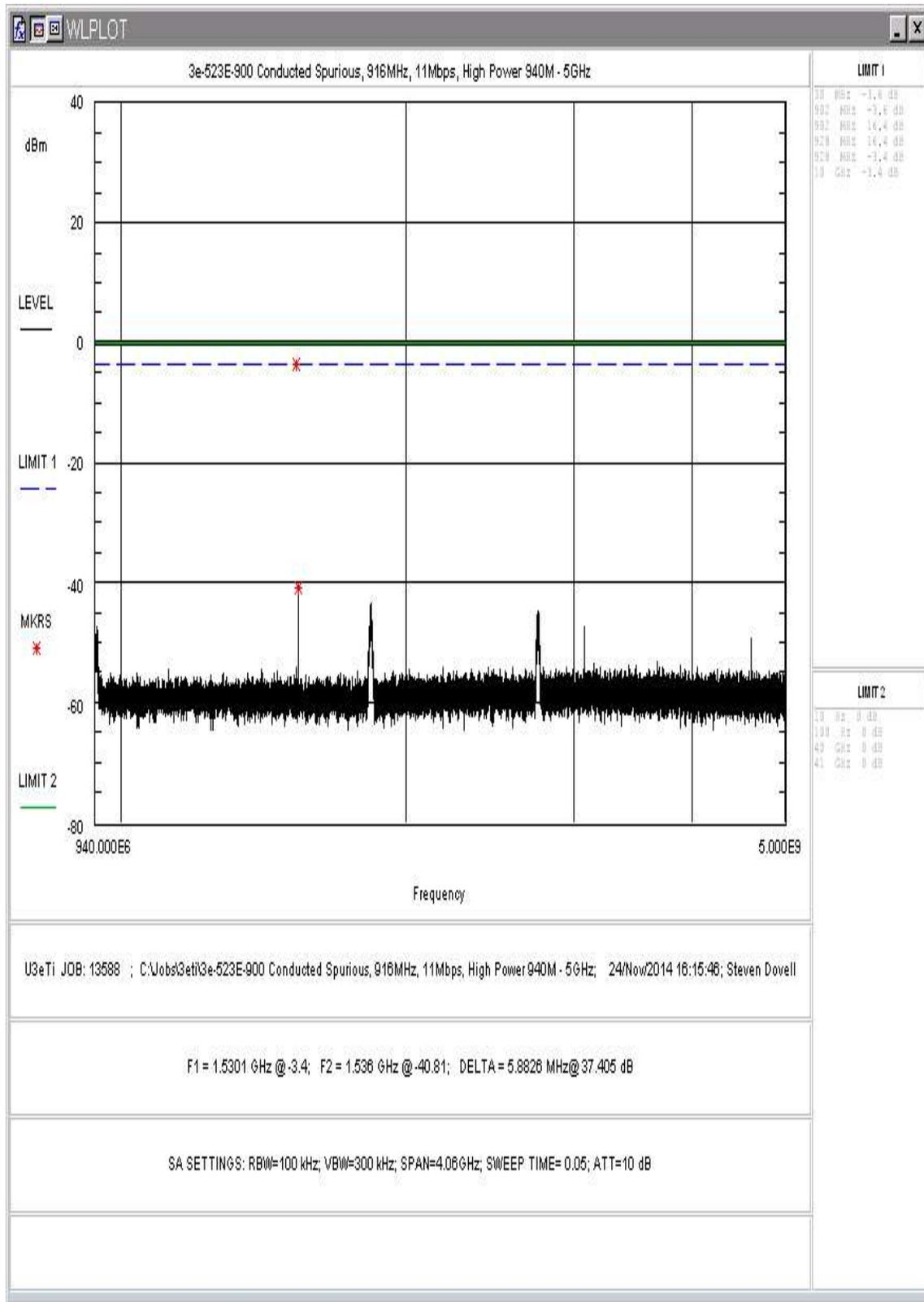
**Figure 11: Conducted Spurious Emissions, 11Mbps, High Power, 940-5000MHz**
