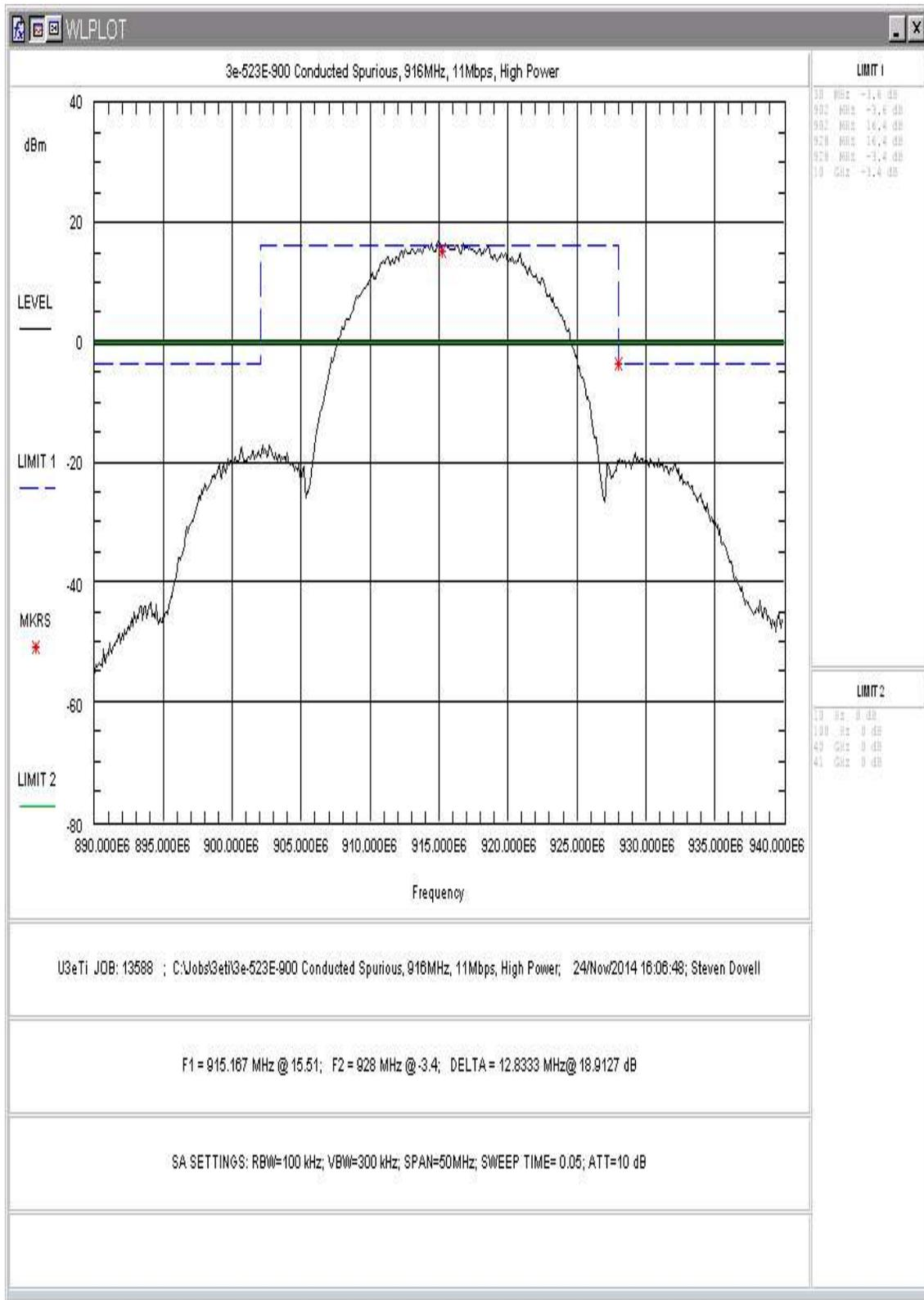
Figure 10: Conducted Spurious Emissions, 11Mbps, High Power, 890-940MHz
