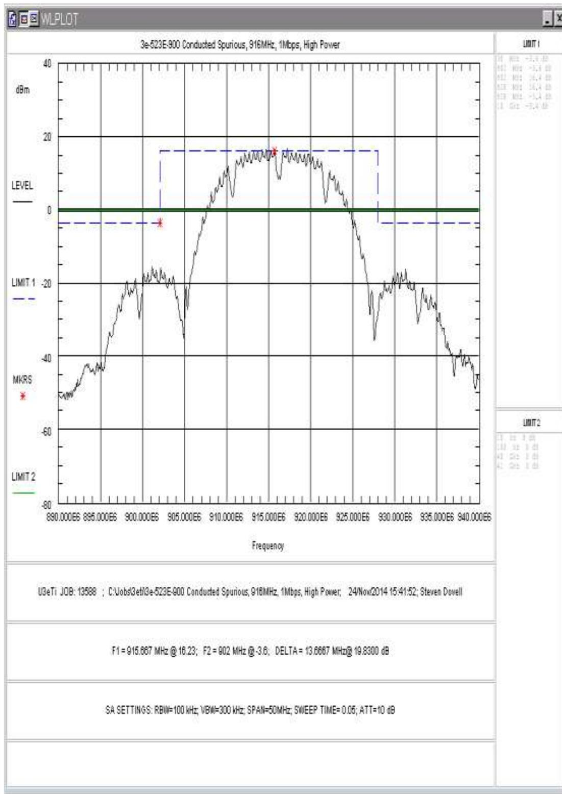
Figure 6: Conducted Spurious Emissions, 1Mbps, High Power, 890 -940MHz
