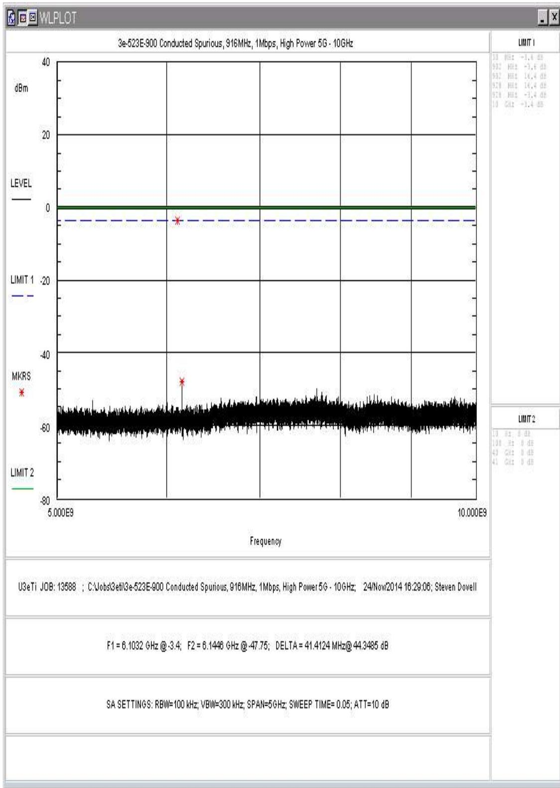
Figure 8: Conducted Spurious Emissions, 1Mbps, High Power, 5 - 10GHz
