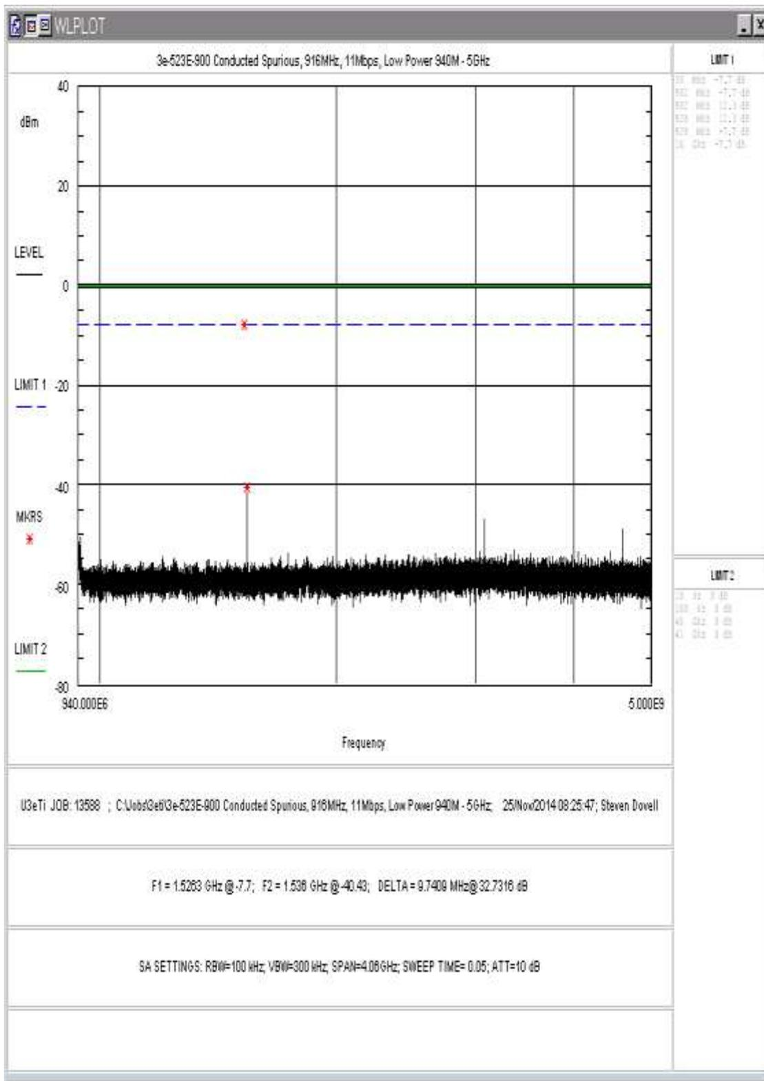
Figure 19: Conducted Spurious Emissions, 11Mbps, Low Power, 940-5000MHz
