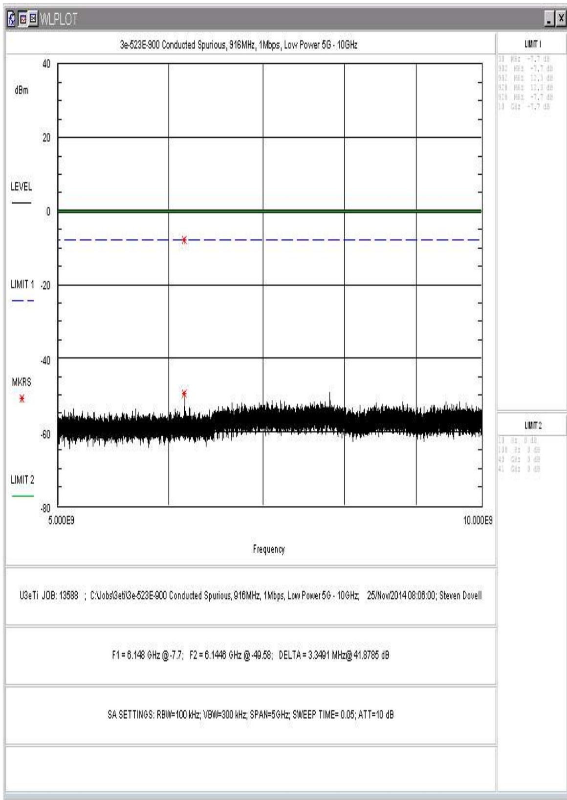
Figure 16: Conducted Spurious Emissions, 1Mbps, Low Power, 5-10GHz
