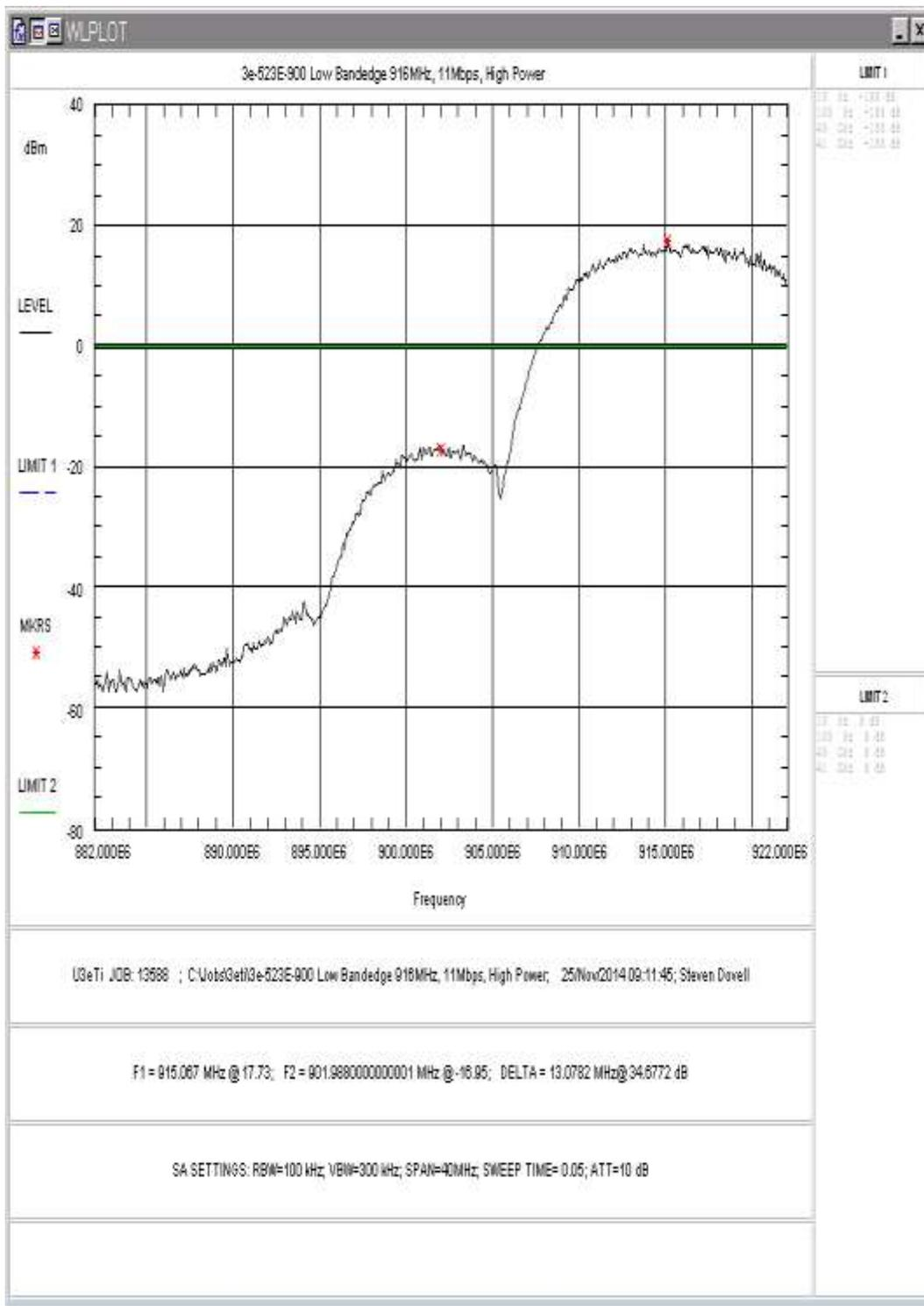
Figure 22: Lower Band-edge, 11Mbps, High Power
