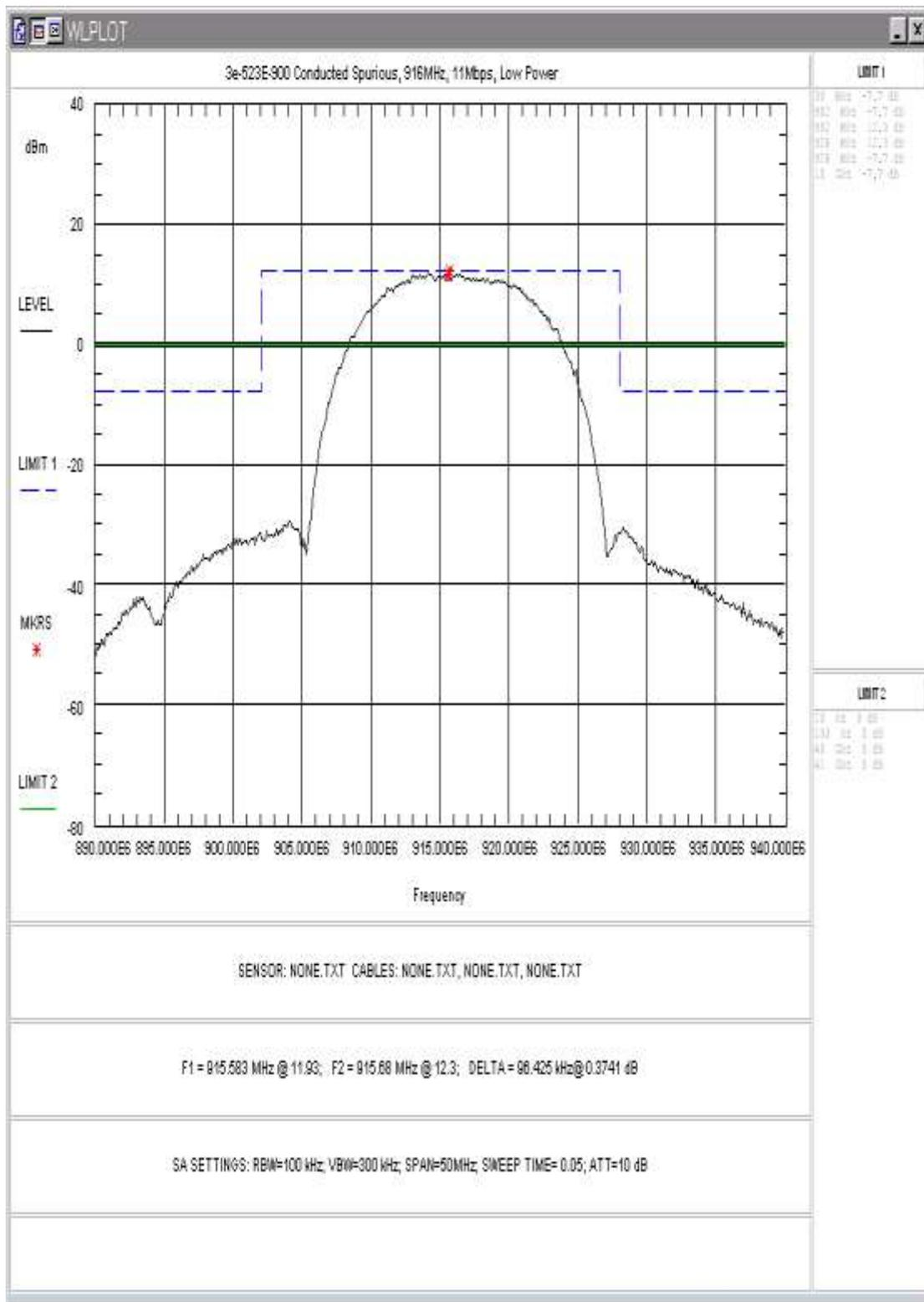
Figure 18: Conducted Spurious Emissions, 11Mbps, Low Power, 890-940MHz
