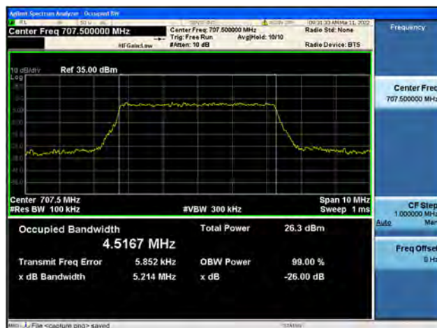
Band12 / 5MHz / Mid CH / 16QAM
