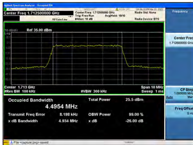
Band4 / 5MHz / Mid CH / 16QAM
