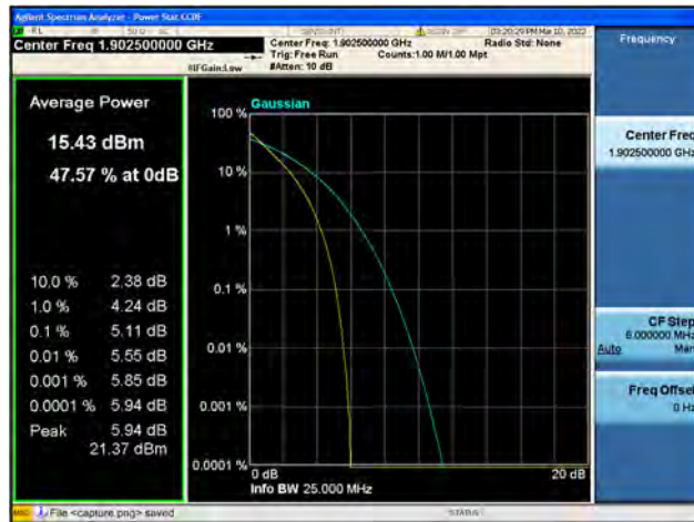
Band2 / 15MHz / High CH / 64QAM
