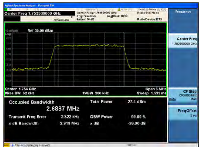
Band4 / 3MHz / High CH / 64QAM
