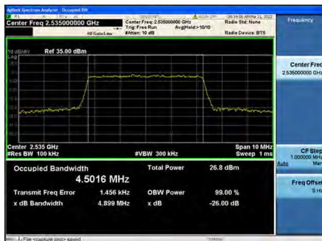
Band7 / 5MHz / Mid CH / 16QAM
