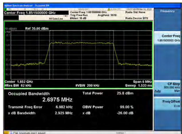
Band2 / 3MHz / Low CH / 64QAM
