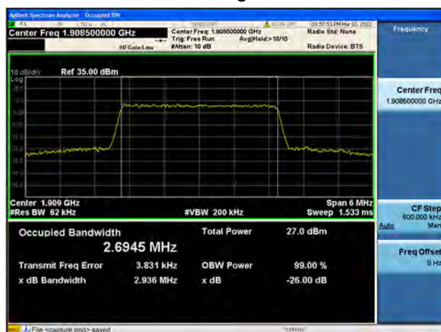
Band2 / 3MHz / High CH / 16QAM
