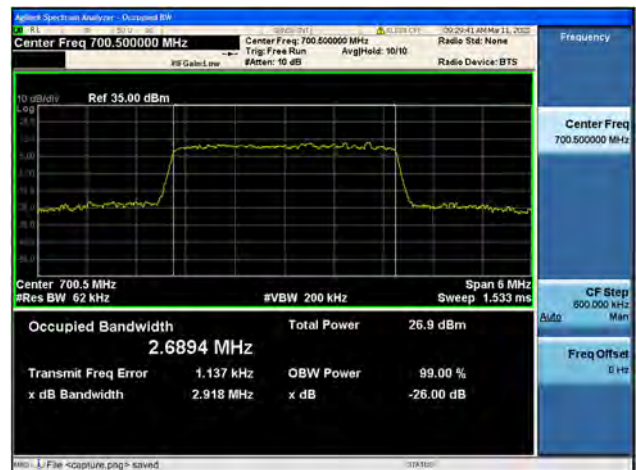
Band12 / 3MHz / Low CH / 64QAM
