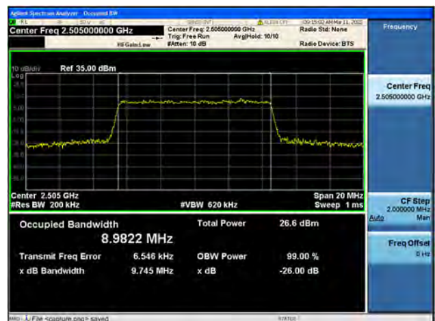
Band7 / 10MHz / Low CH / 64QAM
