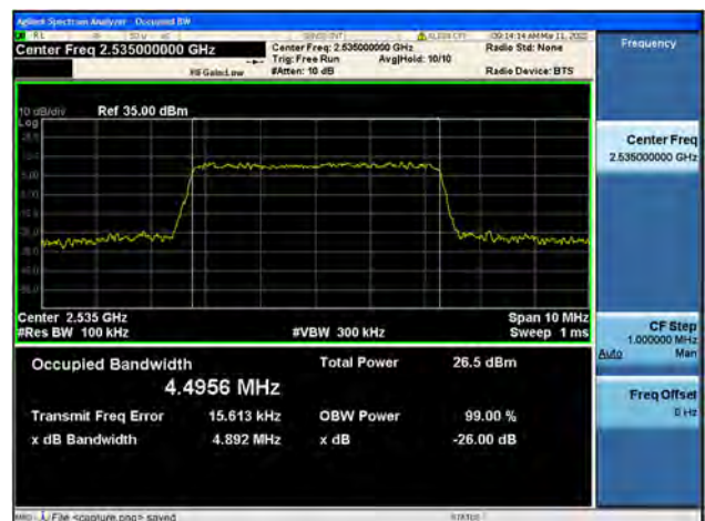
Band7 / 5MHz / Mid CH / 64QAM
