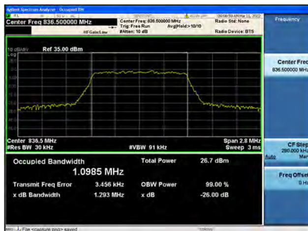
Band5 / 1.4MHz / Mid CH / 16QAM
