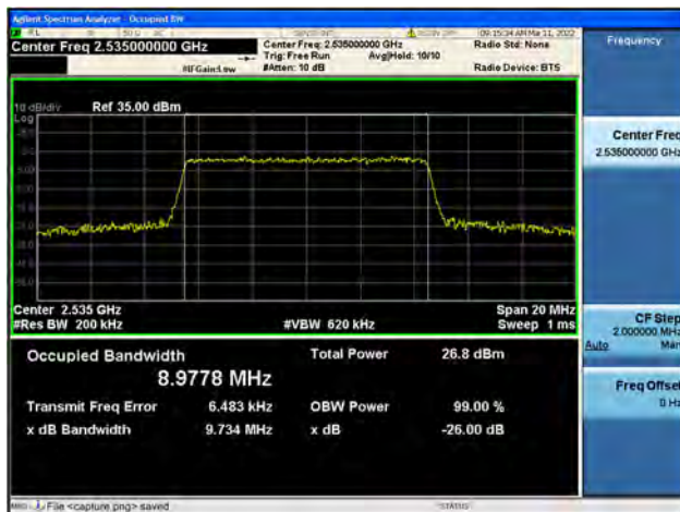
Band7 / 10MHz / High CH / 16QAM
