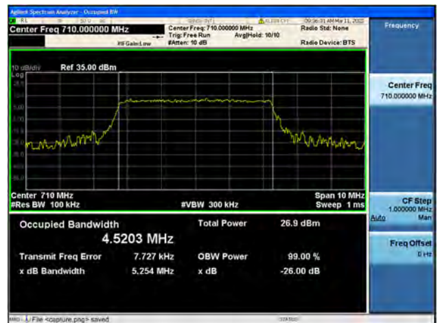
Band17 / 5MHz / Mid CH / 64QAM
