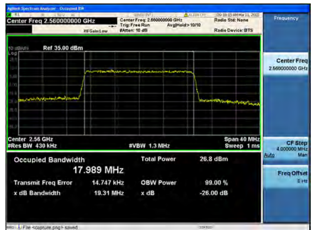
Band7 / 20MHz / High CH / 64QAM
