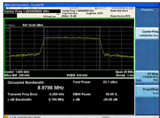
Band2 / 10MHz / High CH / 64QAM
