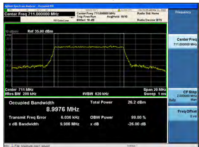
Band12 / 10MHz / High CH / 64QAM
