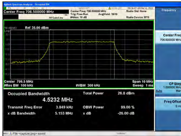
Band17 / 5MHz / Low CH / 64QAM
