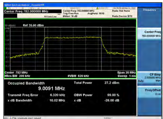
Band13 / 10MHz / High CH / 64QAM
