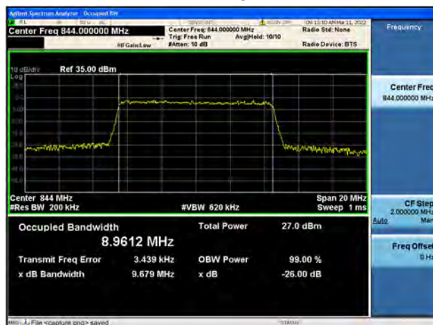
Band5 / 10MHz / High CH / 16QAM
