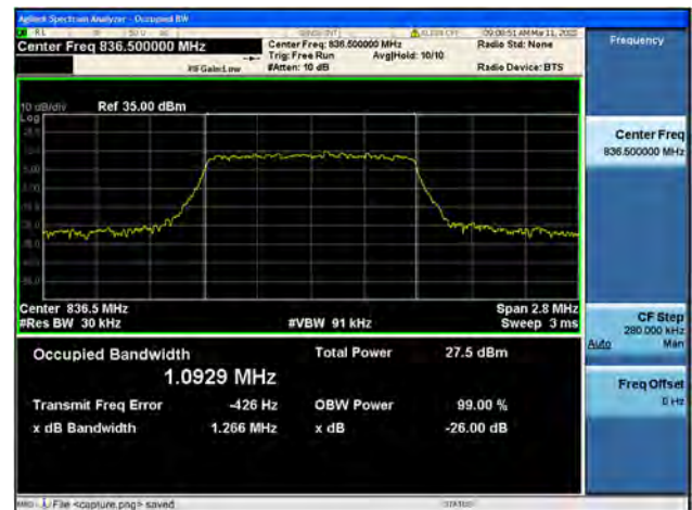
Band5 / 1.4MHz / Mid CH / 64QAM
