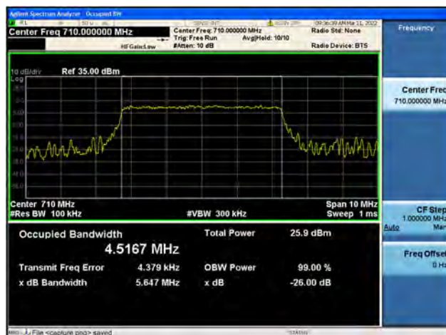
Band17 / 5MHz / Mid CH / 16QAM
