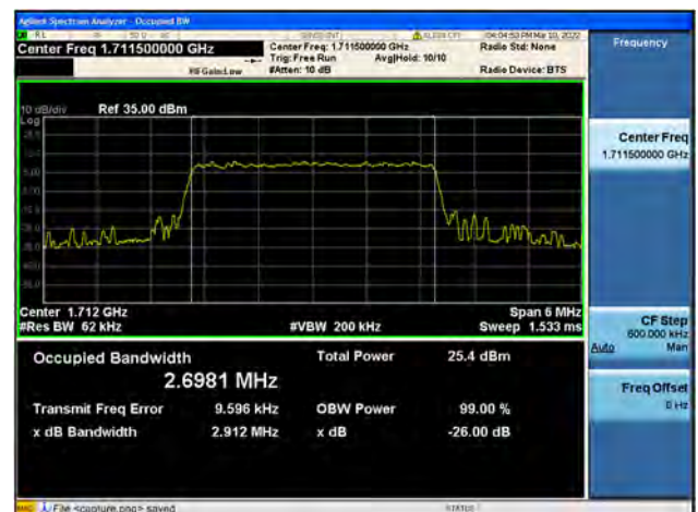
Band4 / 3MHz / Low CH / 64QAM
