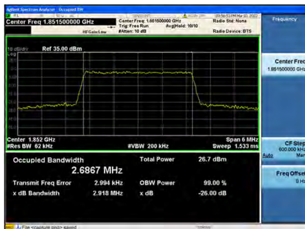
Band2 / 3MHz / Low CH / 16QAM
