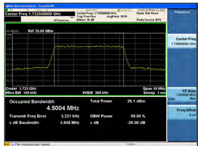
Band4 / 5MHz / Mid CH / 64QAM
