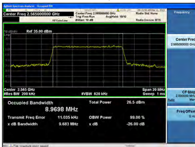
Band7 / 10MHz / High CH / 16QAM
