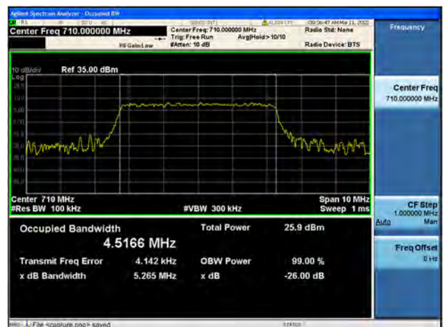
Band17 / 5MHz / Mid CH / 64QAM
