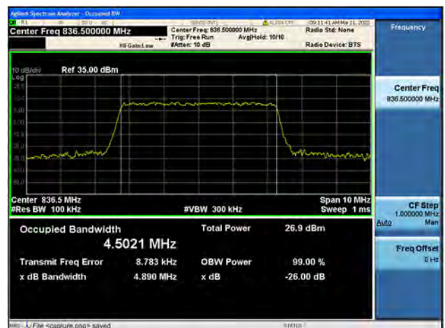
Band5 / 5MHz / Mid CH / 64QAM
