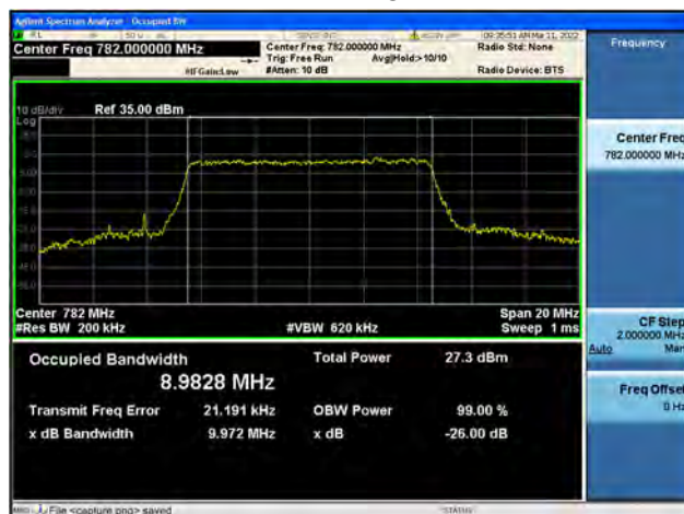
Band13 / 10MHz / High CH / 16QAM
