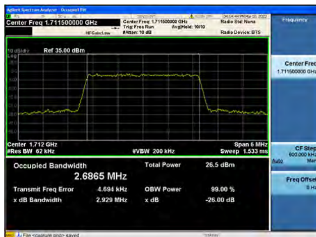
Band4 / 3MHz / Low CH / 16QAM
