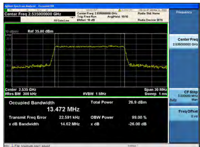
Band7 / 15MHz / Mid CH / 64QAM
