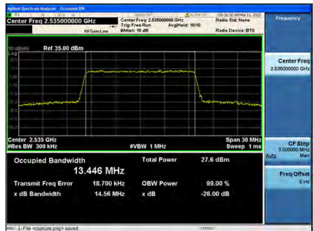
Band7 / 15MHz / Mid CH / 64QAM
