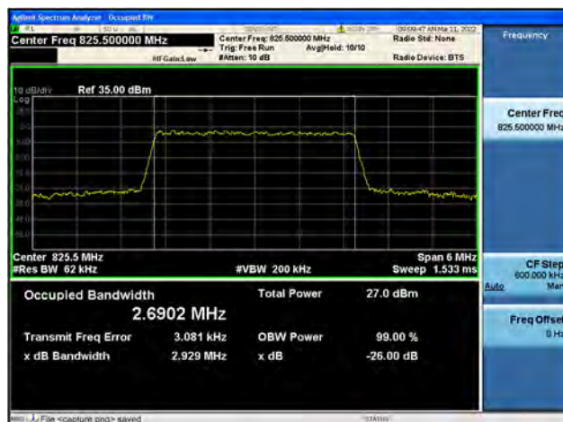
Band5 / 3MHz / Low CH / 16QAM
