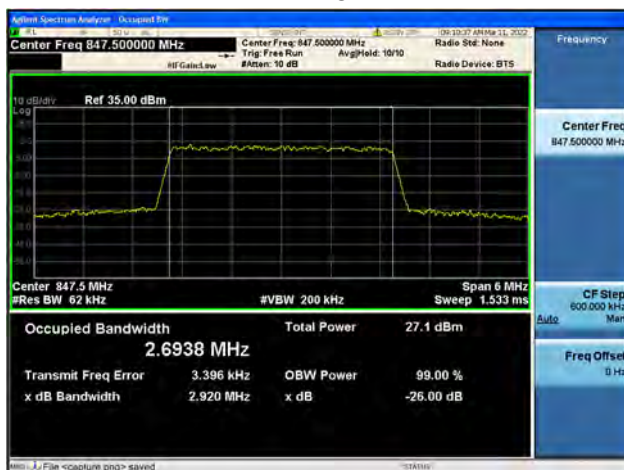
Band5 / 3MHz / High CH / 16QAM
