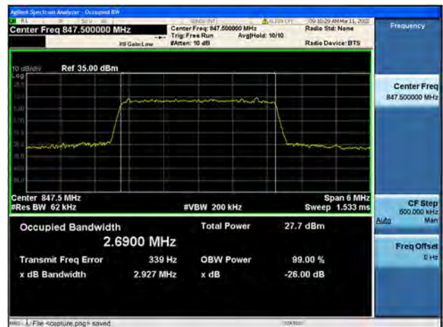
Band5 / 3MHz / High CH / 64QAM
