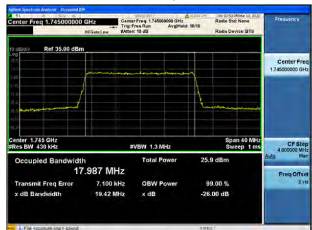
Band4 / 20MHz / High CH / 64QAM
