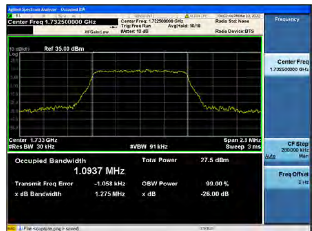
Band4 / 1.4MHz / Mid CH / 64QAM
