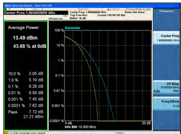
Band2 / 10MHz / High CH / 64QAM
