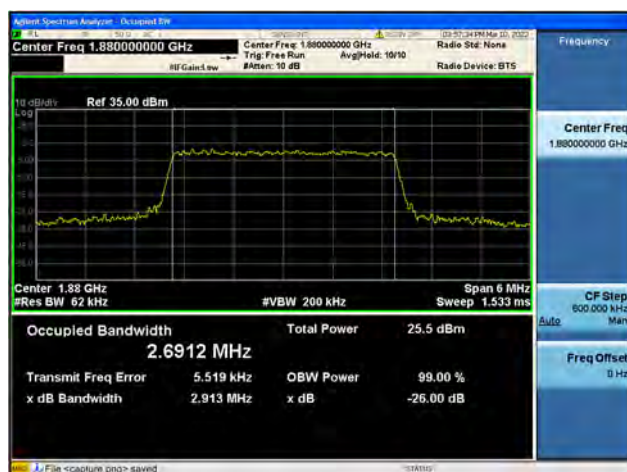
Band2 / 3MHz / High CH / 16QAM
