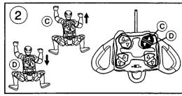
Right arm control: press button C to move the right arm up and press button D to move the right arm down. (See diagram)
