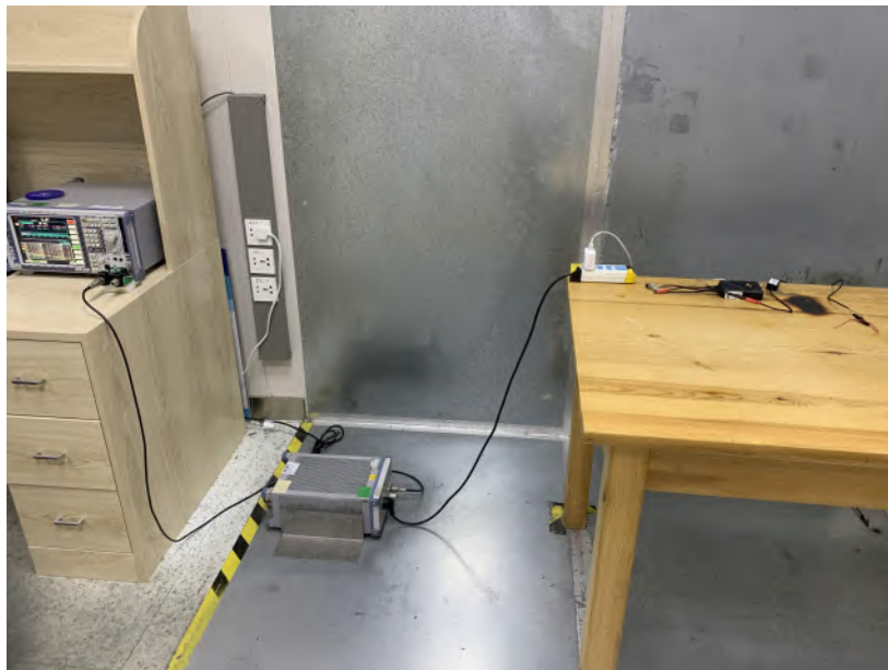
Radiated Spurious Emissions From 30MHz-1000MHz
