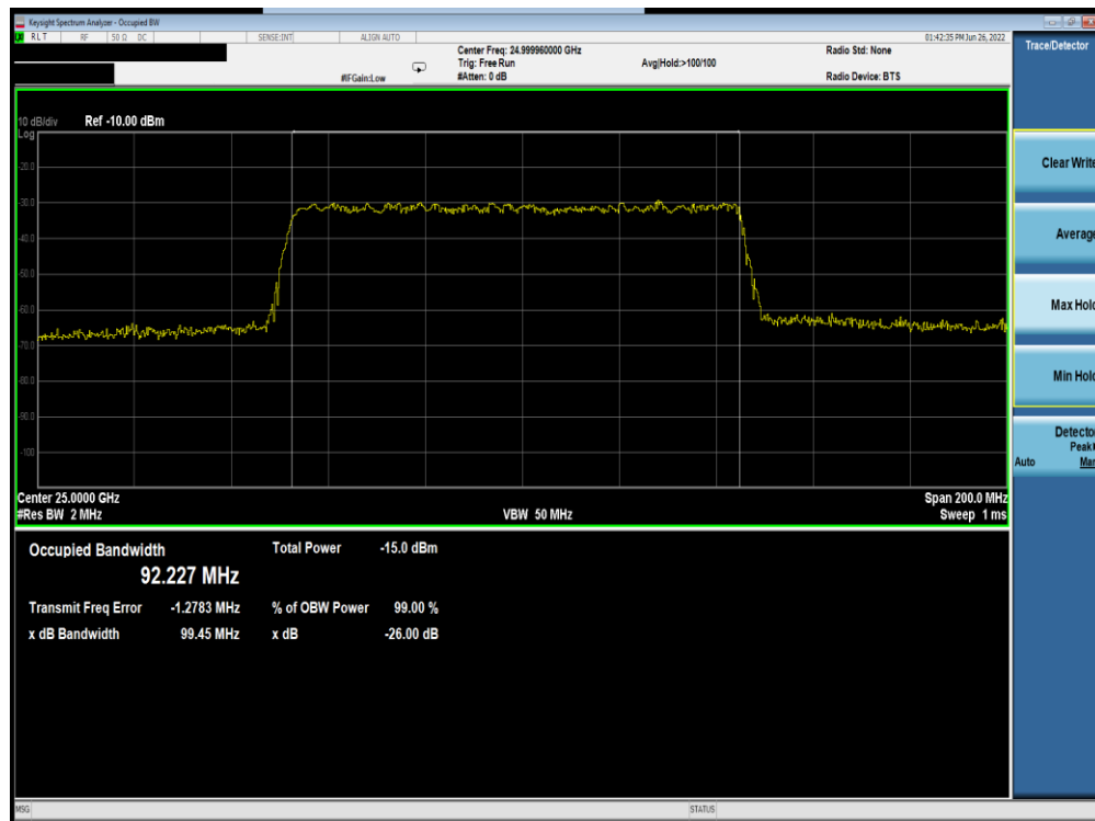
Plot 7-146. Ant M0 OBW (Band n258-R2-100MHz-1CC SISO DFTs-OFDM – 16QAM – Mid Channel)
