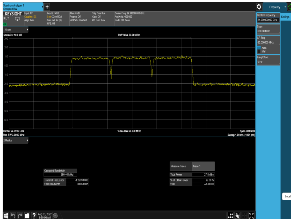
Plot 7-172. Ant M0 OBW (Band n258-R2-100MHz-3CC SISO DFTs-OFDM – \pi/2 BPSK – Mid Channel)
