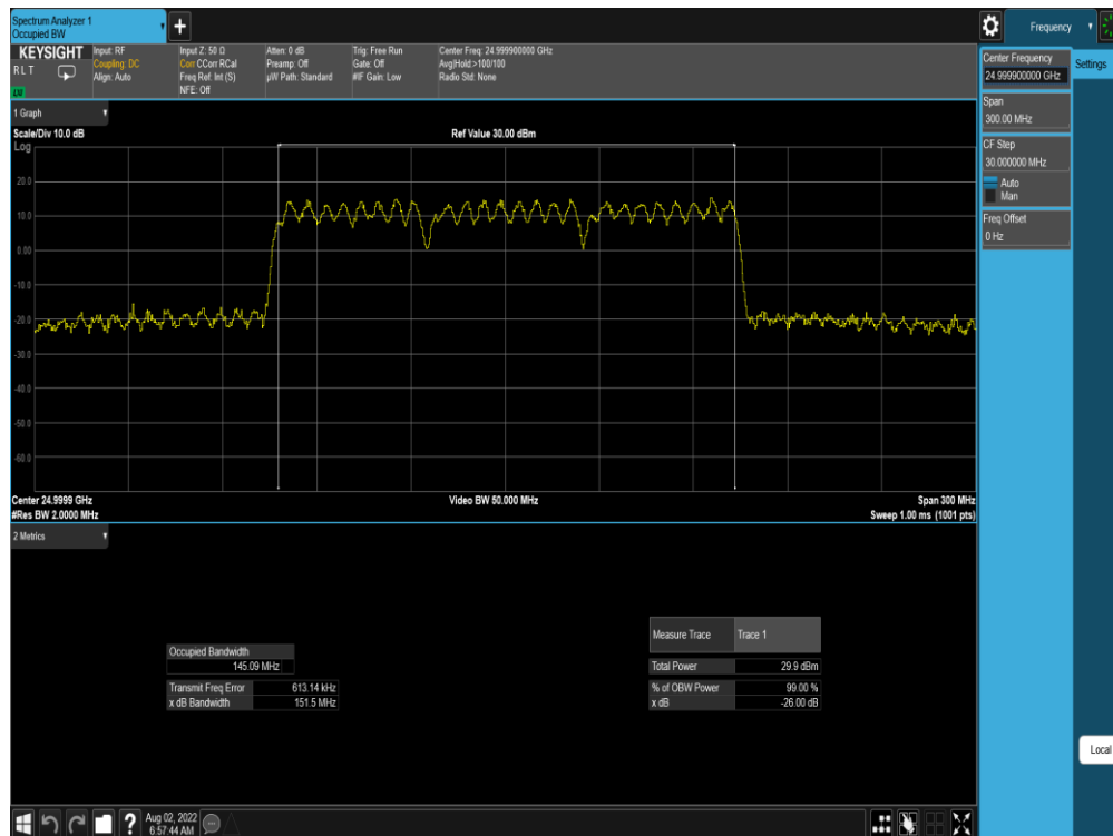
Plot 7-120. Ant M0 OBW (Band n258-R2-50MHz-3CC MIMO CP-OFDM – QPSK – Mid Channel)
