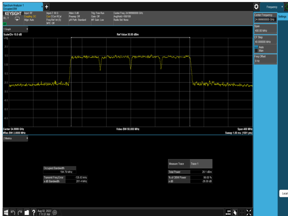
Plot 7-132. Ant M0 OBW (Band n258-R2-50MHz-4CC SISO DFTs-OFDM – 16QAM – Mid Channel)
