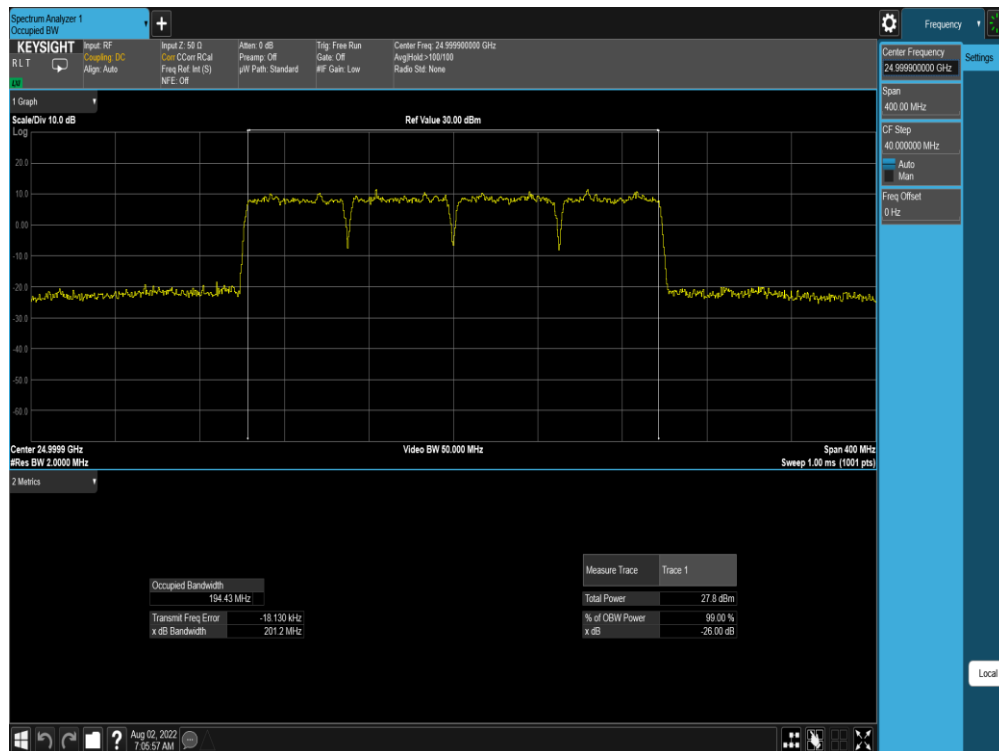
Plot 7-130. Ant M0 OBW (Band n258-R2-50MHz-4CC SISO DFTs-OFDM – \pi/2 BPSK – Mid Channel)
