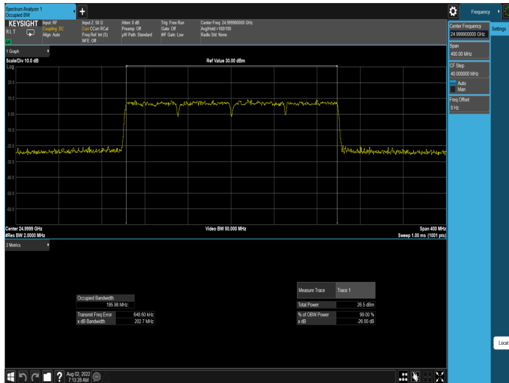
Plot 7-129. Ant M0 OBW (Band n258-R2-50MHz-4CC SISO CP-OFDM – 64QAM – Mid Channel)
