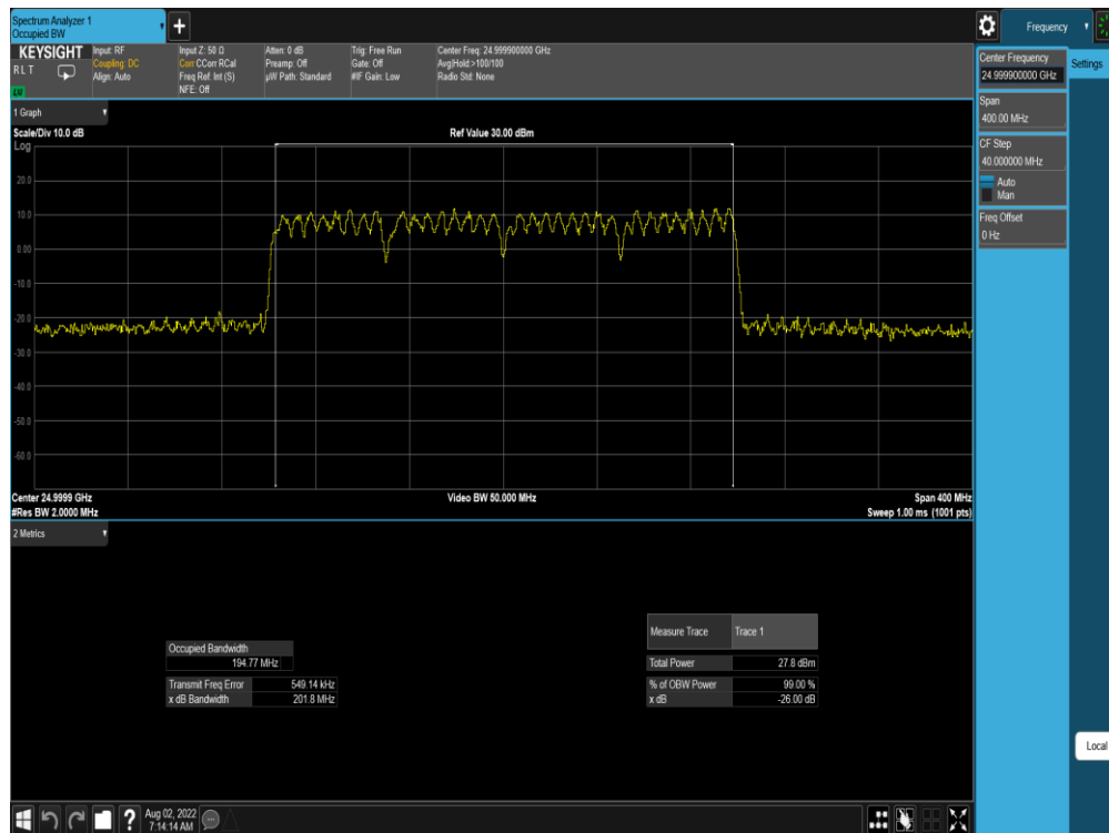
Plot 7-136. Ant M0 OBW (Band n258-R2-50MHz-4CC MIMO CP-OFDM – 64QAM – Mid Channel)
