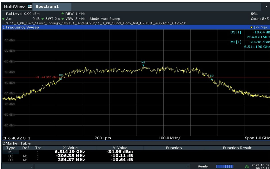
Plot 7-10. 10dBc Bandwidth – CH.5 - SP0 – Preamble 12
