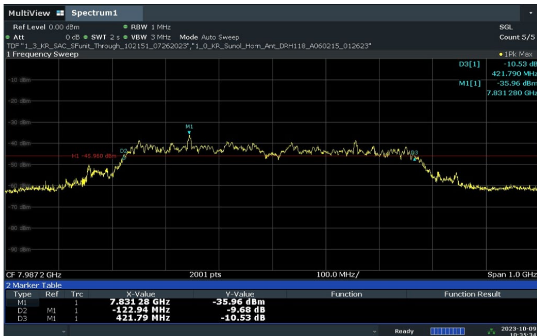
Plot 7-16. 10dBc Bandwidth – CH.9 - SP0 – Preamble 9
