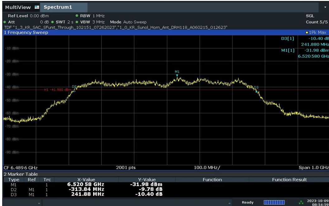
Plot 7-3. 10dBc Bandwidth – CH.5 – SP3 – Preamble 9
