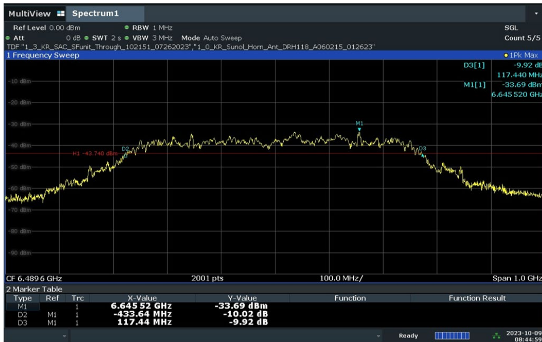
Plot 7-1. 10dBc Bandwidth – CH.5 - SP0 – Preamble 9
