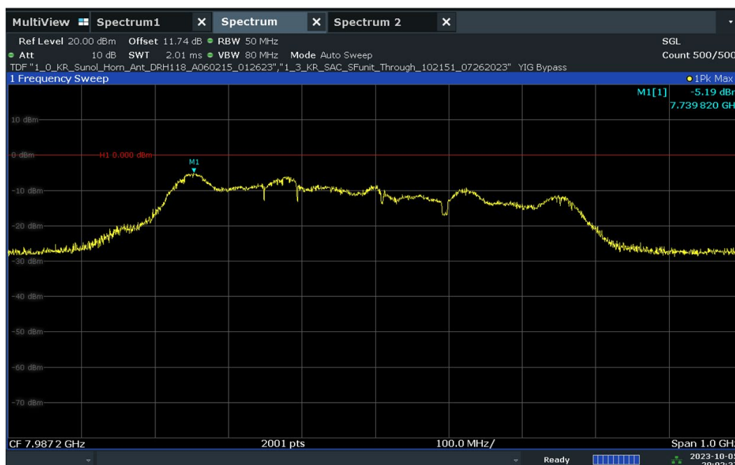
Plot 7-37. UWB Peak Power Measurement - CH.9 – HPRF
