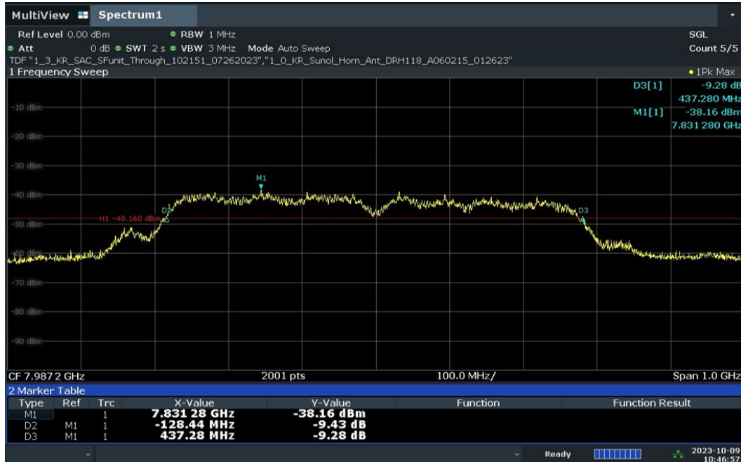
Plot 7-27. 10dBc Bandwidth – CH.9 – SP3 – Preamble 12
