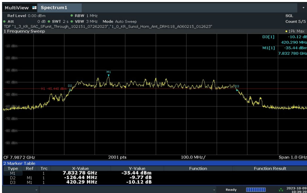
Plot 7-20. 10dBc Bandwidth – CH.9 – SP1 – Preamble 10
