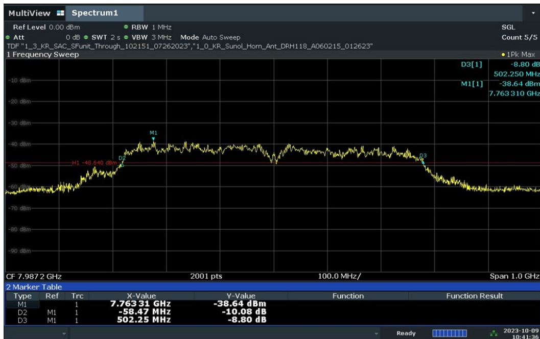
Plot 7-22. 10dBc Bandwidth – CH.9 - SP0 – Preamble 11
