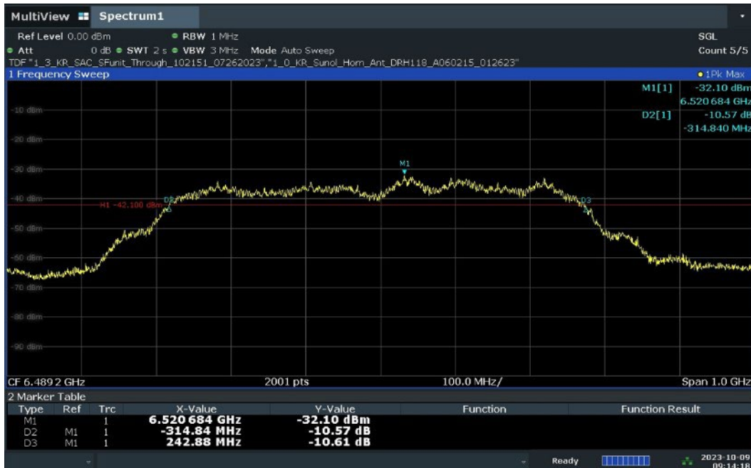
Plot 7-9. 10dBc Bandwidth – CH.5 – SP3 – Preamble 11
