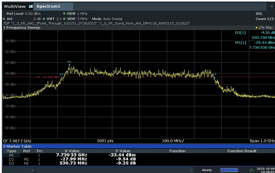
Plot 7-28. 10dBc Bandwidth – CH.9 - SP0 – Preamble 27
