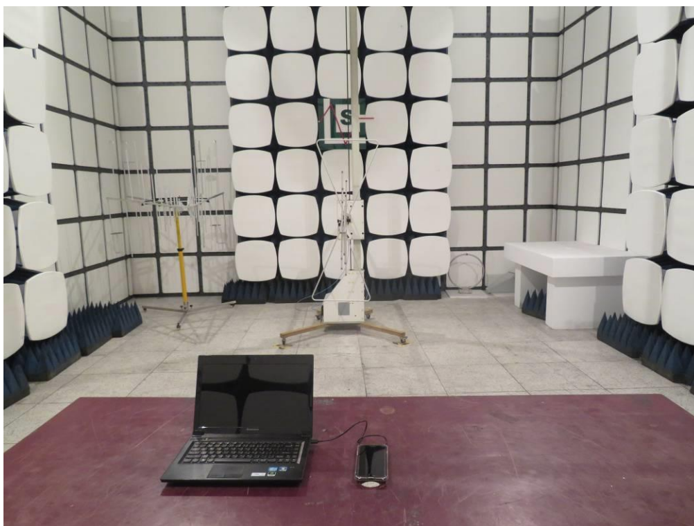
Radiated Emission below 1GHz-PC charge mode
