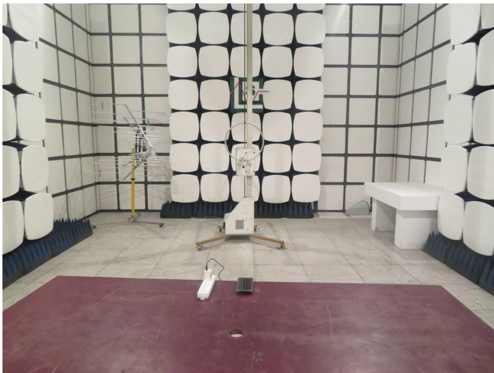
Radiated Emission below 30MHz-AC adapter charge mode
