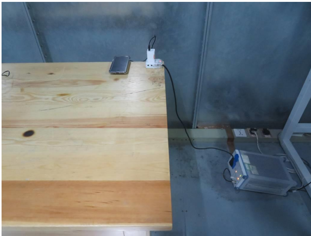
Conducted Emission-AC adapter charge mode
