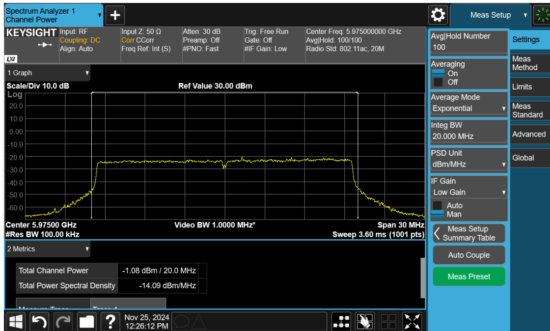
Plot 17: Power and PSD for Low-Power Indoor – 5975 MHz
