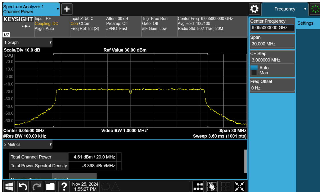
Plot 21: Power and PSD for Standard Power– 6055 MHz
