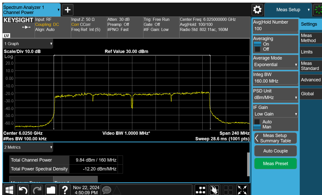
Plot 11: Power and PSD for Standard Power – 6025 MHz
