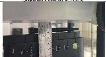
Back Side and Ant Vertical (Separation distance of 10mm)
