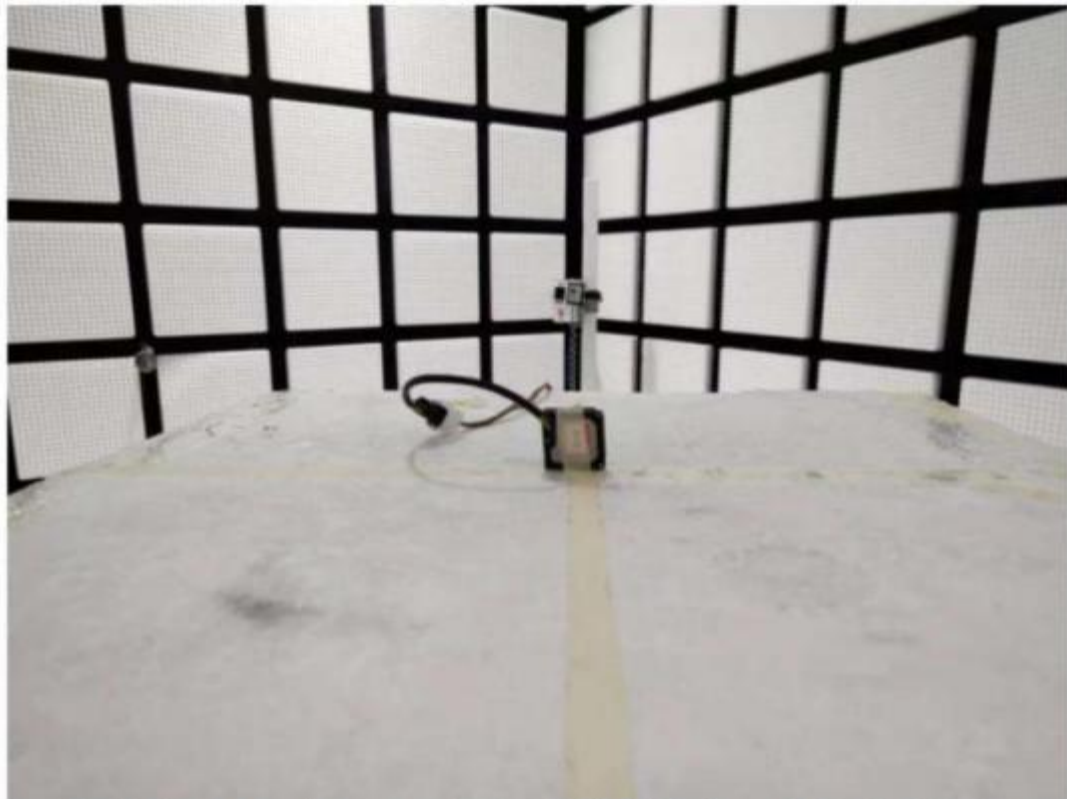
Radiated spurious emission Test Setup-3(18GHz-41GHz)
