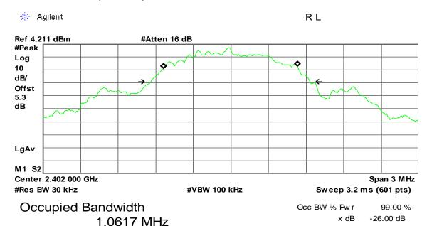
Transmit Freq Error -2.881 kHz x dB Bandw idth 1.272 MHz
