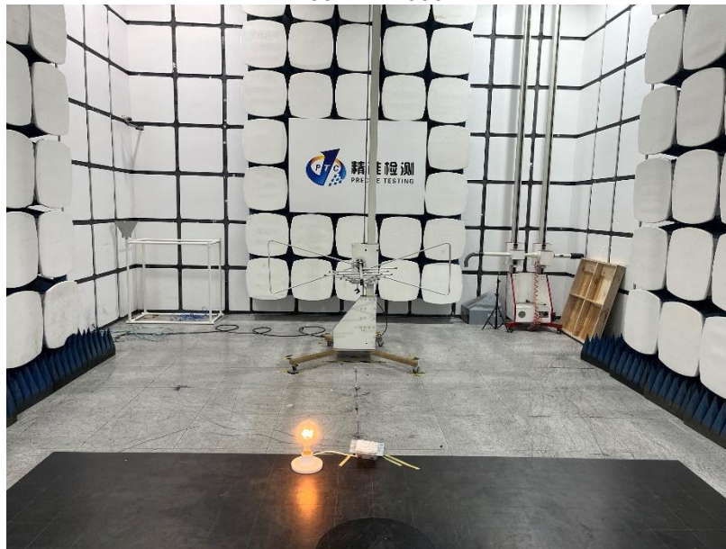
Radiated Spurious Emissions From 30MHz-1000MHz
