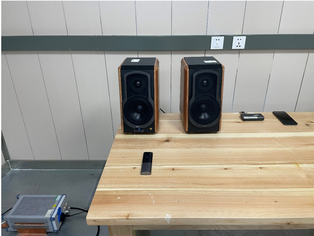
Photograph 1: Set-up for Conducted Emission on AC Mains
