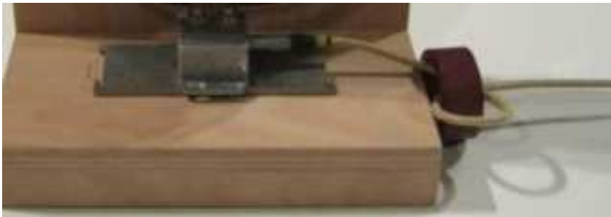
Fig. 4.3: EMI suppressor at stator unit
