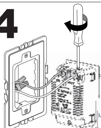
Connect new device as shown. Make sure the terminal holes are clear. Insert wires into terminals and tighten screws securely. Do NOT over-tighten. (to 10 in. lbs.)
