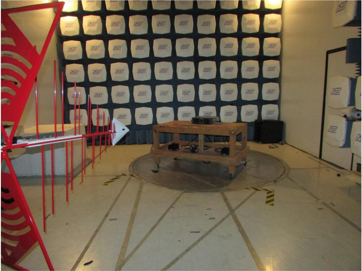
30-1000MHz Radiated Measurements
