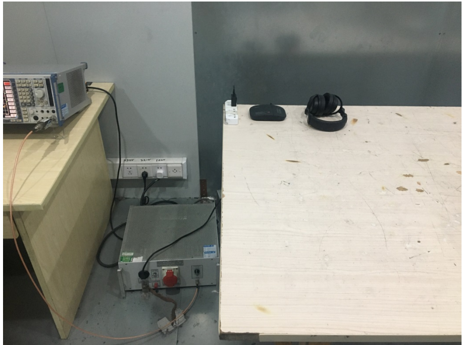
Conducted Emission Test Setup
