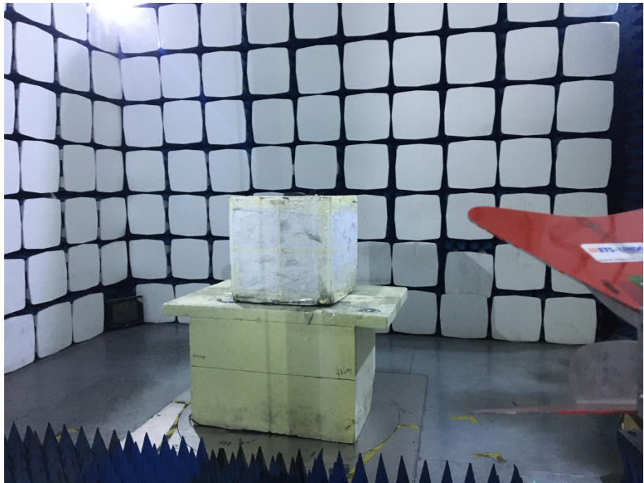
Radiation Emission Test Setup (1GHz to 18GHz)
