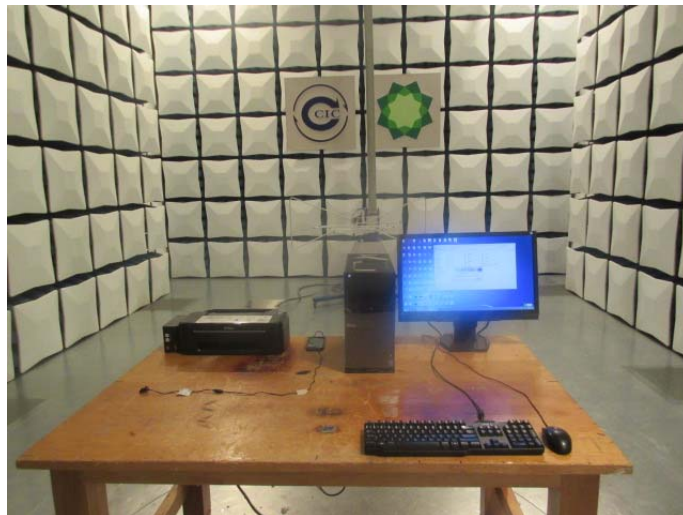
Radiated Emission (above 1GHz) Connect to PC
