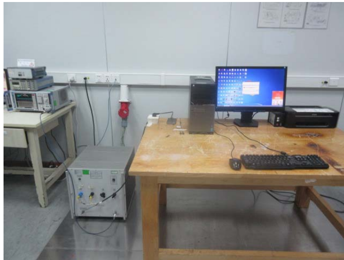
Radiated Emission (30MHz-1GHz) Connect to PC
