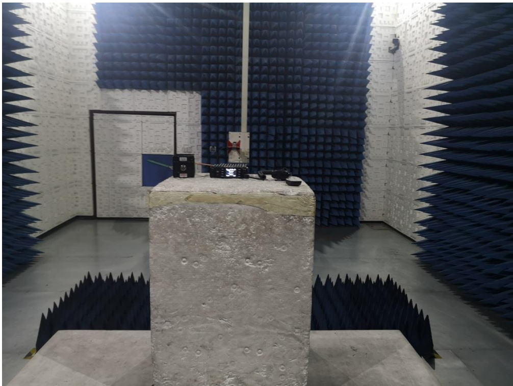
RADIATED EMISSION TEST SETUP ABOVE 1GHz
