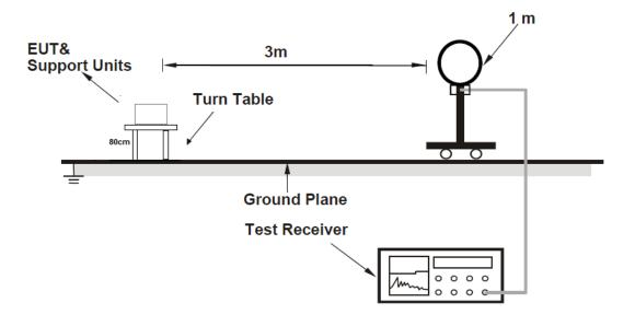
For Radiated emission between 30MHz~1000MHz
