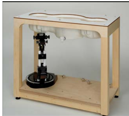
Picture C.10: SAM Twin Phantom
