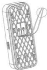
Step 5. Mount your Smart Doorbell on the Bracket with Security Screws ;
