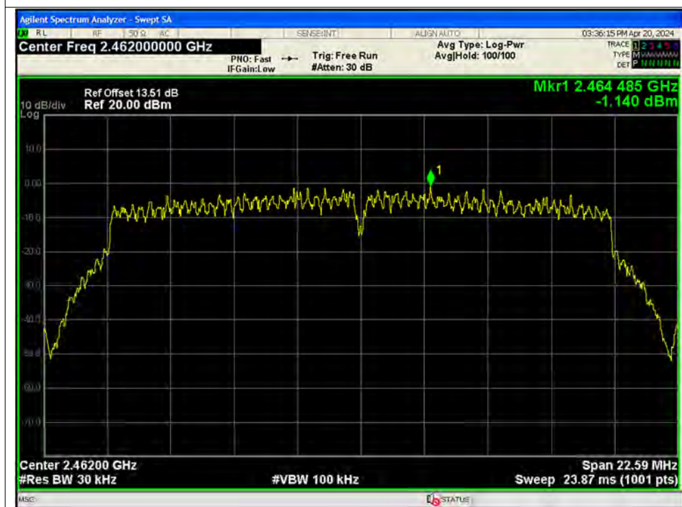
PSD NVNT n20 2462MHz Ant2 MIMO
