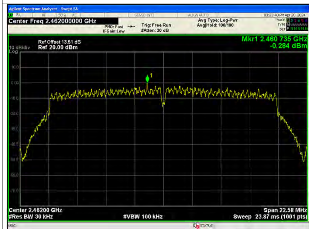
PSD NVNT n20 2462MHz Ant2 SISO
