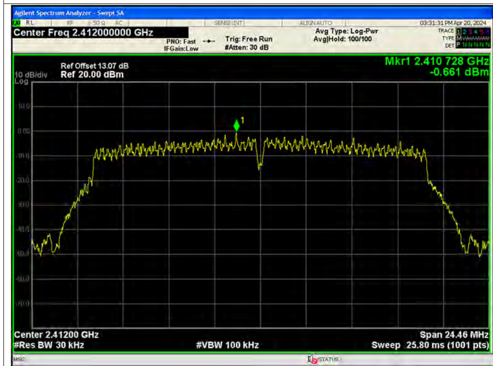
PSD NVNT n20 2412MHz Ant2 MIMO
