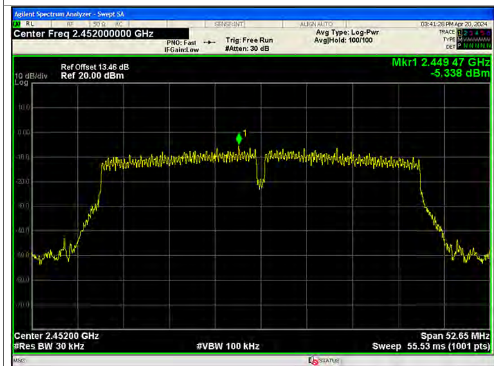
PSD NVNT n40 2452MHz Ant2 MIMO
