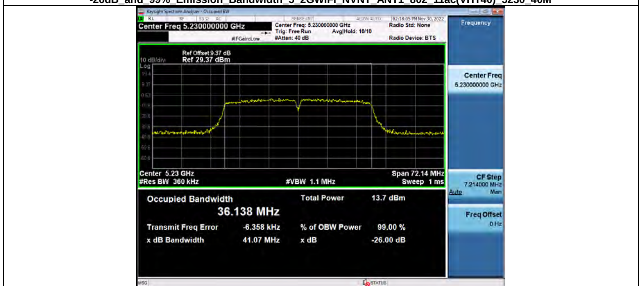
-26dB and 99% Emission Bandwidth 5 2GWiFi_NVNT_ANT1_802_11ac(VHT80)_5210_80M
