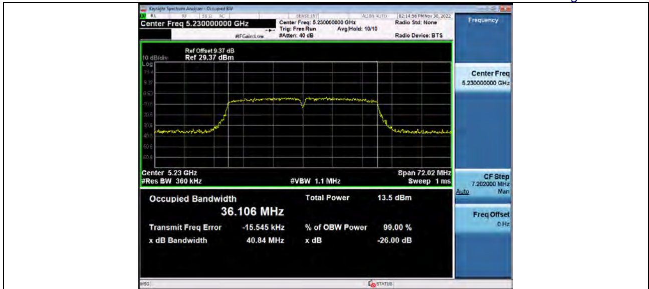
-26dB and 99% Emission Bandwidth 5 2GWiFi_NVNT_ANT1_802_11ac(VHT40)_5190_40M
