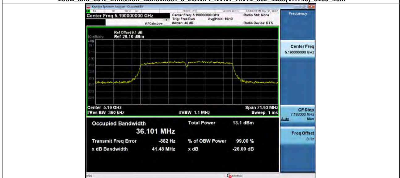
-26dB and 99% Emission Bandwidth 5 2GWiFi_NVNT_ANT1_802_11ac(VHT40)_5190_40M
