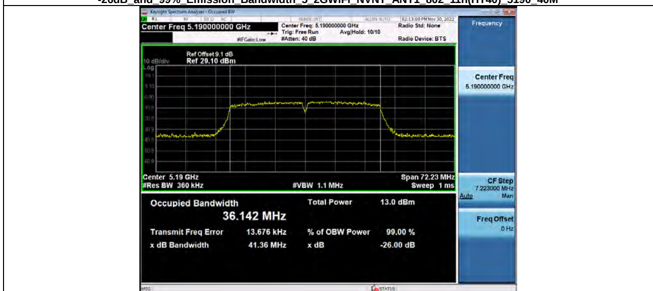
-26dB and 99% Emission Bandwidth 5 2GWiFi_NVNT_ANT1_802_11n(HT40)_5230_40M
