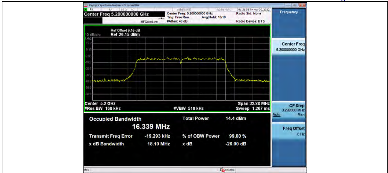
-26dB and 99% Emission Bandwidth 5_2GWiFi_NVNT_ANT1_802_11a_5240_20M
