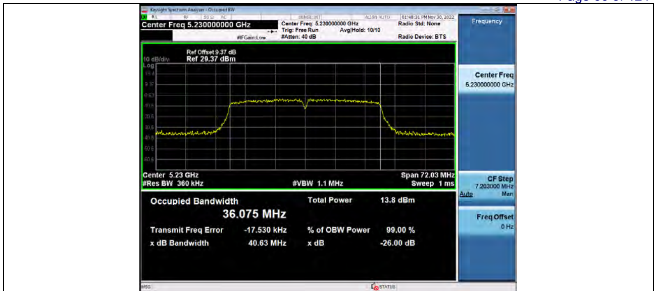
-26dB_and_99% Emission Bandwidth 5 2GWiFi_NVNT_ANT1_802_11ac(VHT40)_5190_40M
