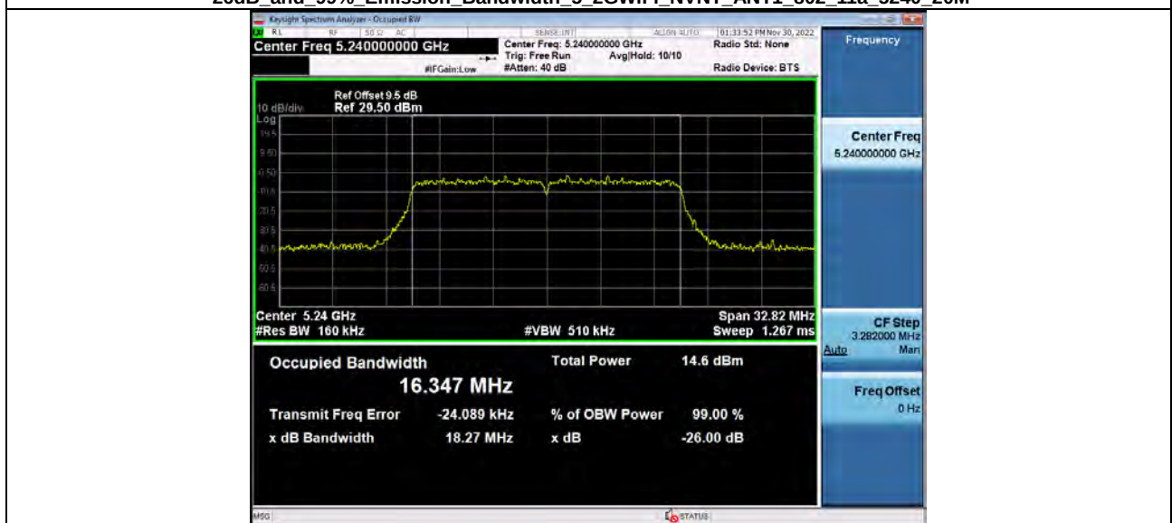
-26dB and 99% Emission Bandwidth 5_2GWiFi_NVNT_ANT1_802_11a_5240_20M
