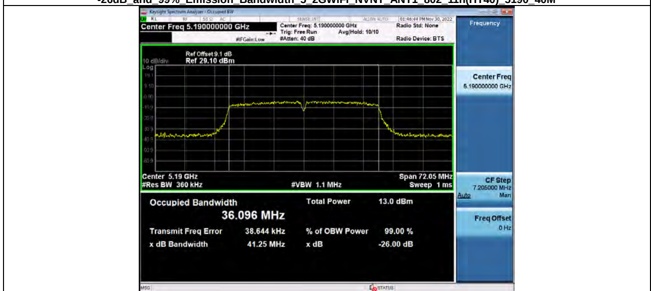
-26dB and 99% Emission Bandwidth 5 2GWiFi_NVNT_ANT1_802_11n(HT40)_5230_40M
