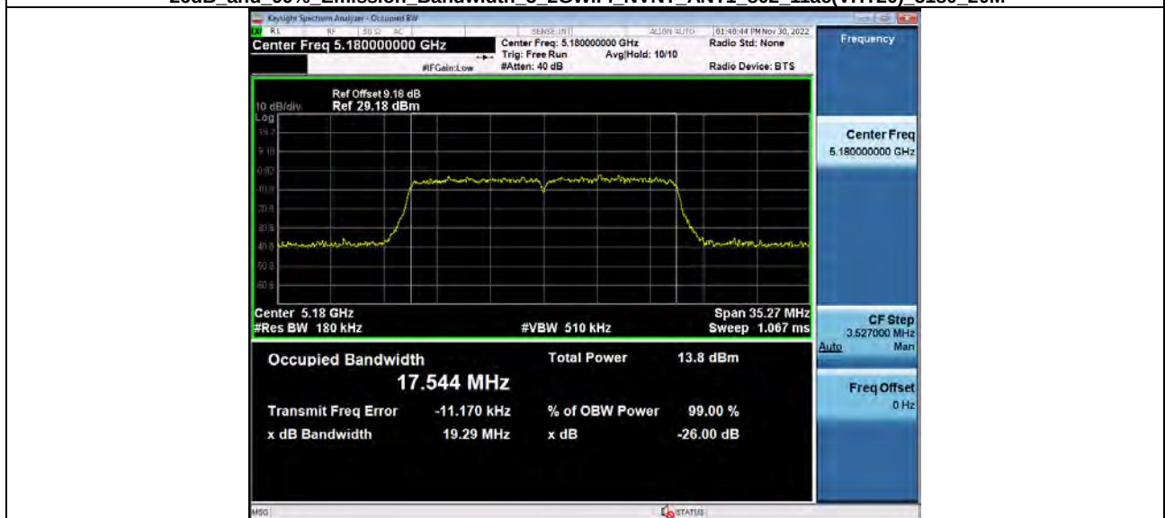
-26dB and 99% Emission Bandwidth 5_2GWiFi_NVNT_ANT1_802_11ac(VHT20)_5180_20M
