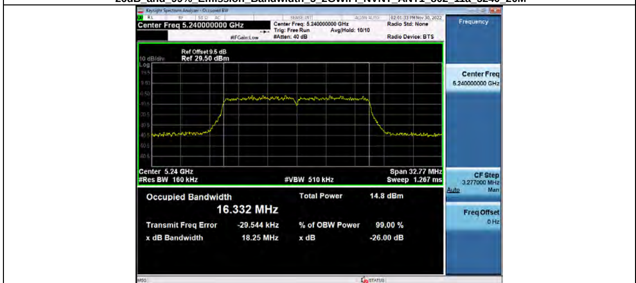
-26dB and 99% Emission Bandwidth 5_2GWiFi_NVNT_ANT1_802_11a_5240_20M
