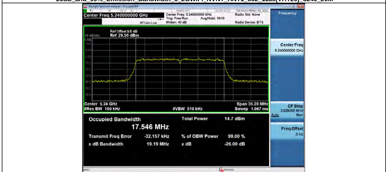
-26dB and 99% Emission Bandwidth 5 2GWiFi_NVNT_ANT1_802_11ac(VHT20)_5240_20M
