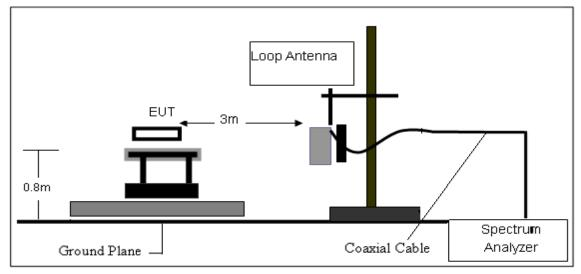
2. Radiated Emission Test-Up Frequency Below1GHz
