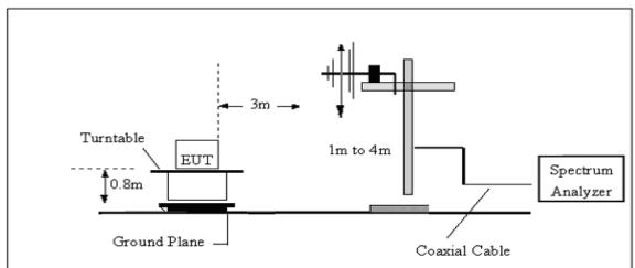
3. Radiated Emission Test-Up Frequency Above 1GHz
