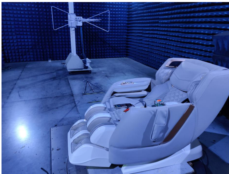
Photo of Radiated Emission Measurement Below 1GHz
