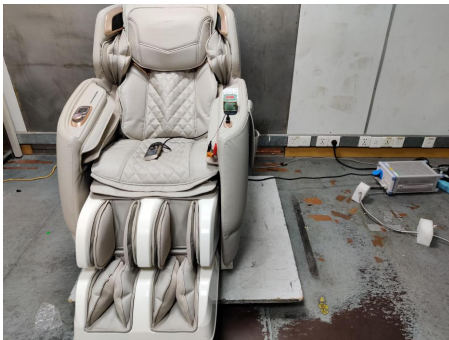
Photo of Power Line Conducted Emission Measurement
