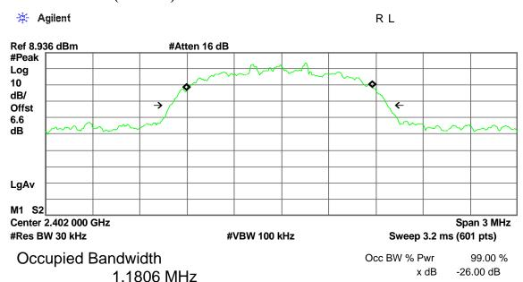
Transmit Freq Error -13.480 kHz x dB Bandwidth 1.384 MHz
