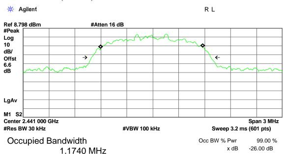
Transmit Freq Error -12.788 kHz x dB Bandwidth 1.383 MHz
