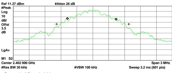
Occupied Bandwidth 919.0859 kHz Occ BW % Pwr 99.00 % x dB -26.00 dB
