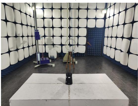
3. Radiated emission (9KHz-30MHz)
