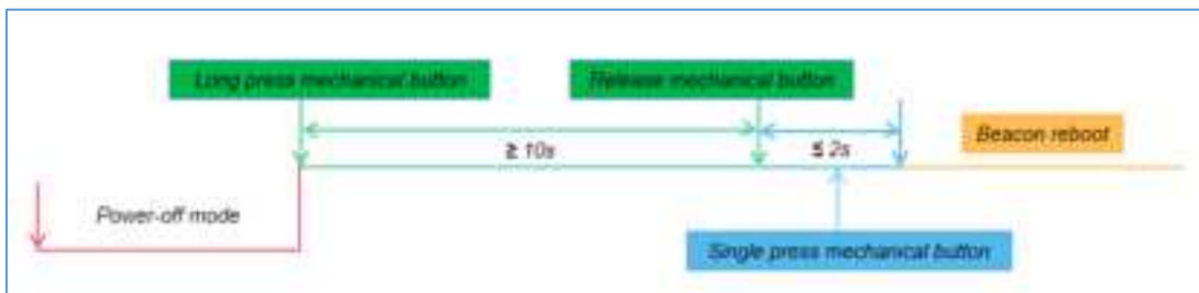
Figure 2: How to reset L03 Series Products
