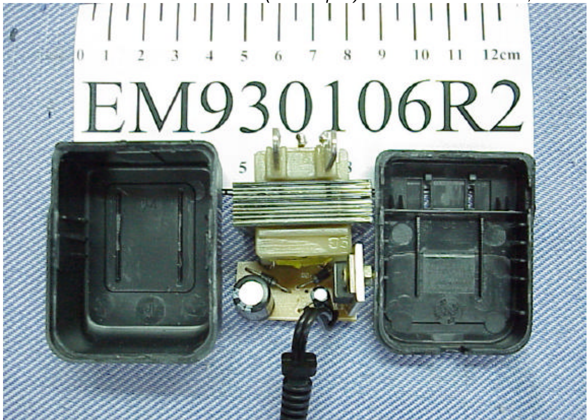
Photo 16 (AC Adapter) Remove Case Covers, Internal View
