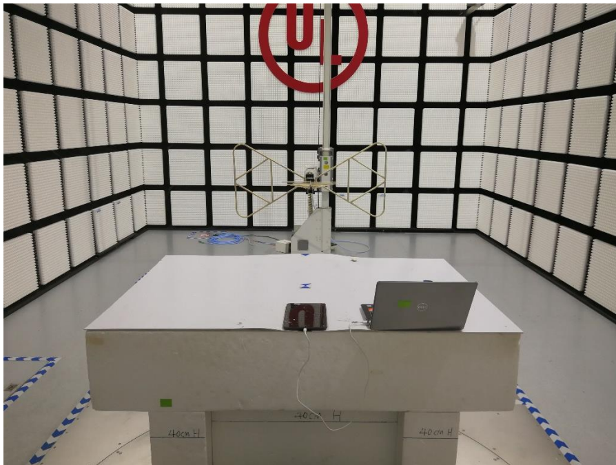
RADIATED RF MEASUREMENT SETUP (30MHz~1GHz)
