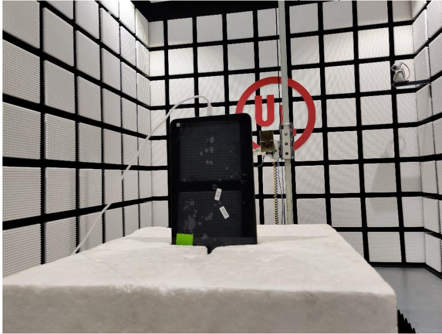
RADIATED RF MEASUREMENT SETUP (30MHz~1GHz)
