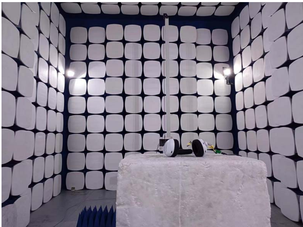
Radiated Setup photo (Above 1G)
