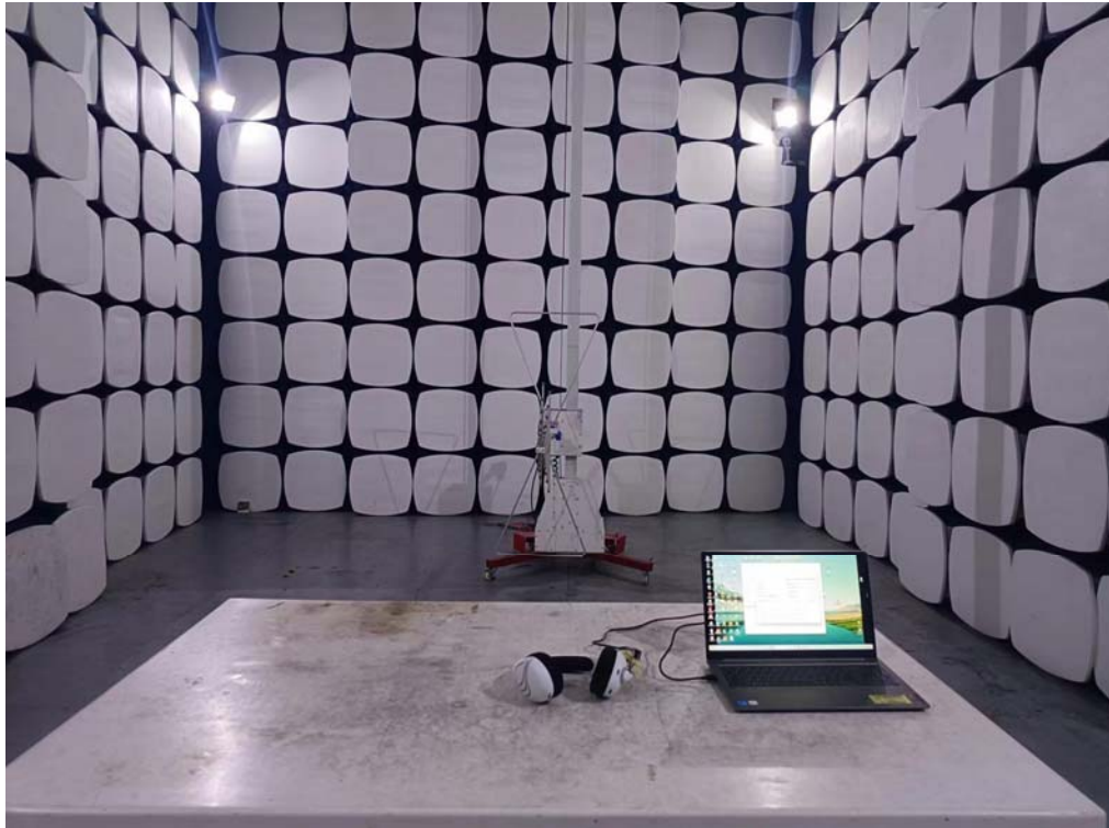
Radiated Setup photo (Below 1G)
