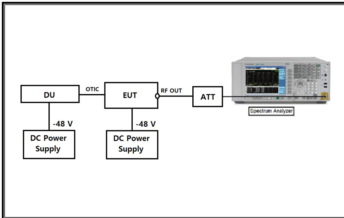
**SETUP DIAGRAM FOR TESTS (RADIATED TEST SETUP)**
