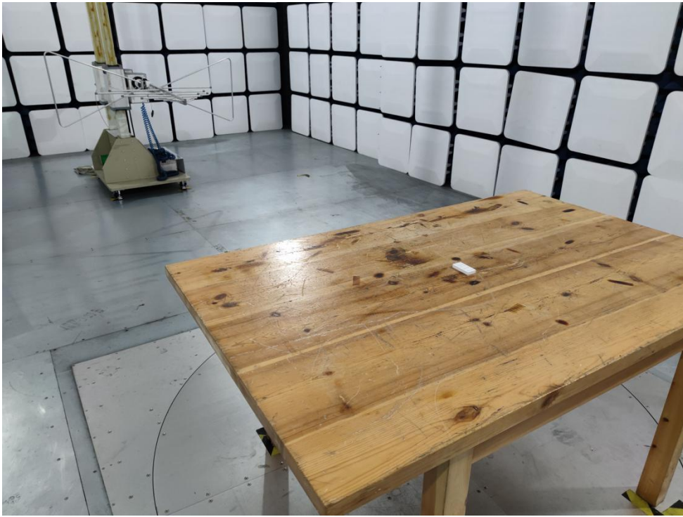
Photo of Radiation Emission Test
