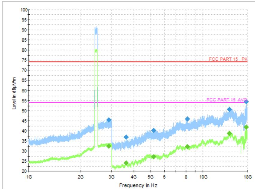
Fig.39 Radiated Spurious Emission (Ch0, 1 GHz - 18 GHz), 1M
