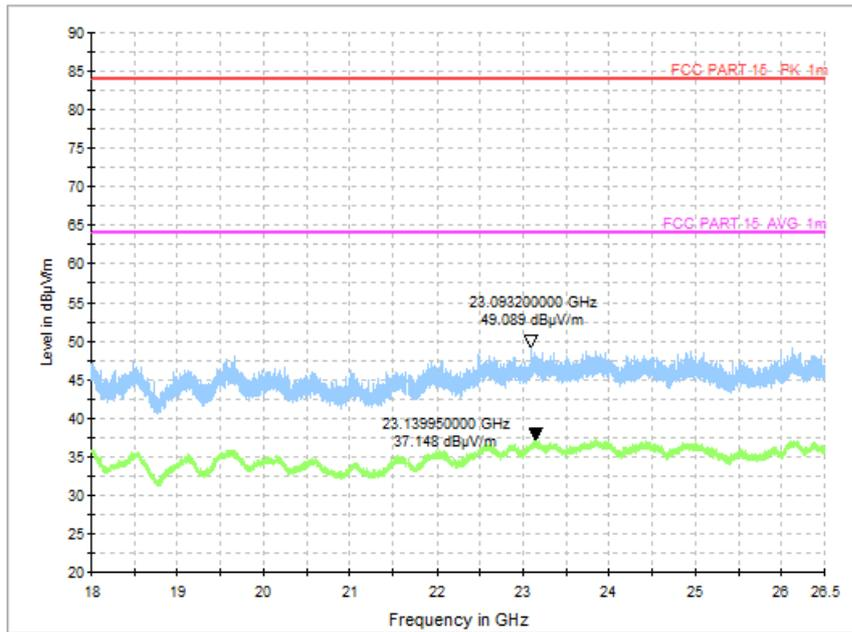
Fig.51 Radiated Spurious Emission (Ch19, 18 GHz - 26.5 GHz), 2M
