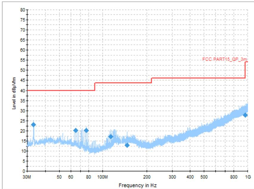
Fig.41 Radiated Spurious Emission (Ch19, 30 MHz - 1 GHz), 1M
