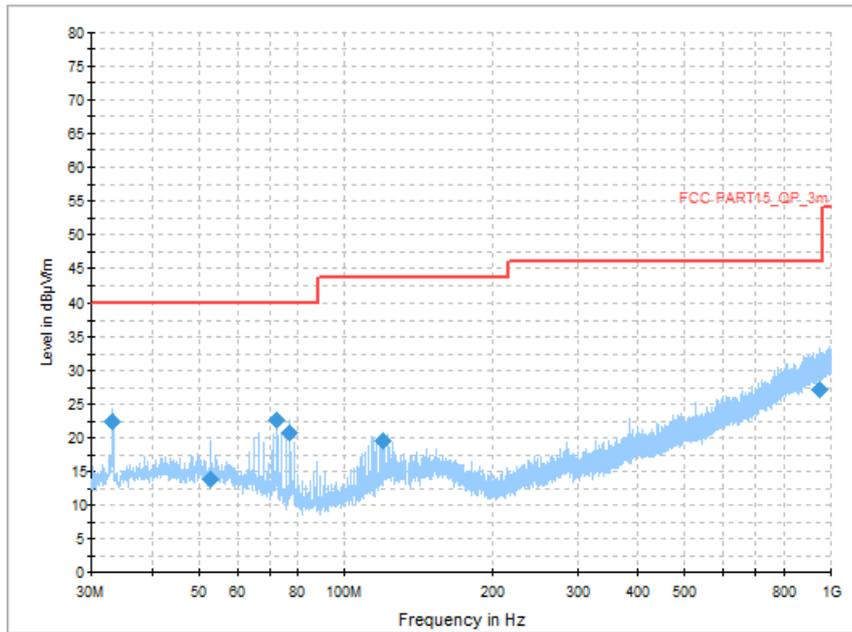
Fig.49 Radiated Spurious Emission (Ch19, 30 MHz - 1 GHz), 2M
