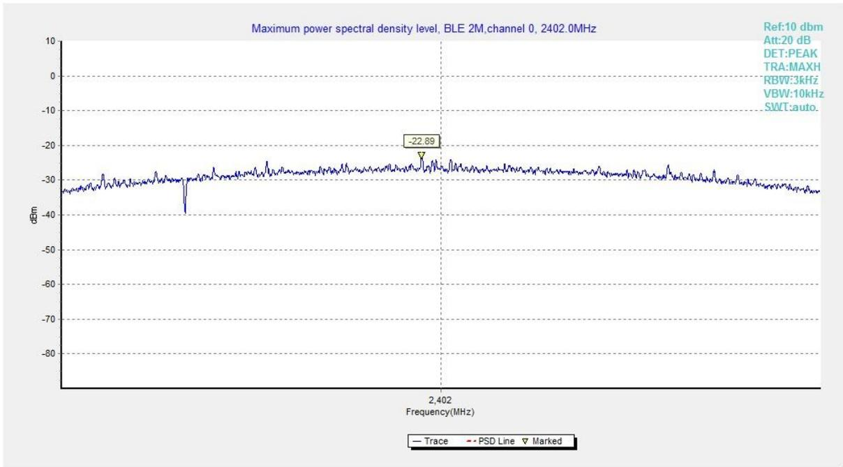
Fig.4 Power Spectral Density (Ch 0), LE 2M
