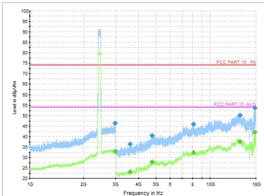
Fig.50 Radiated Spurious Emission (Ch19, 1 GHz - 18 GHz), 2M
