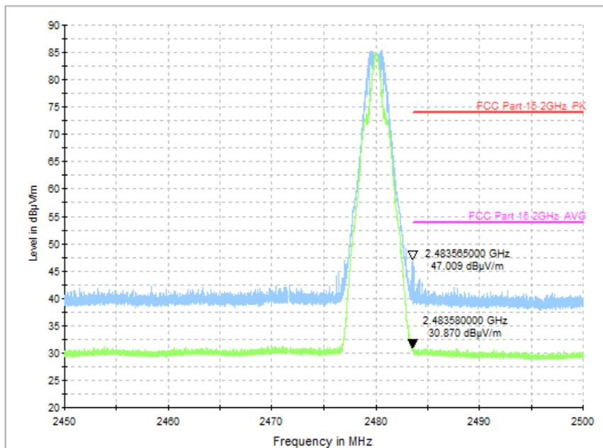
Fig.54 Radiated Band Edges (Ch39, 2450GHz - 2500GHz), 2M
