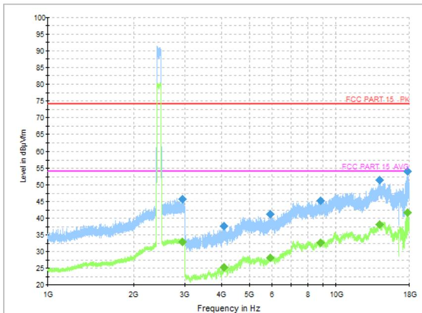
Fig.44 Radiated Spurious Emission (Ch39, 1 GHz - 18 GHz), 1M
