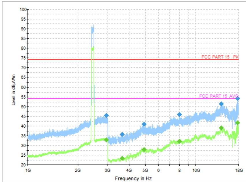
Fig.47 Radiated Spurious Emission (Ch0, 1 GHz - 18 GHz), 2M
