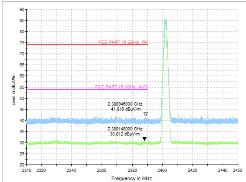
Fig.53 Radiated Band Edges (Ch0, 2380GHz - 2450GHz), 2M
