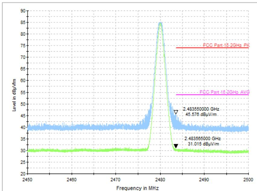
Fig.46 Radiated Band Edges (Ch39, 2450GHz - 2500GHz), 1M
