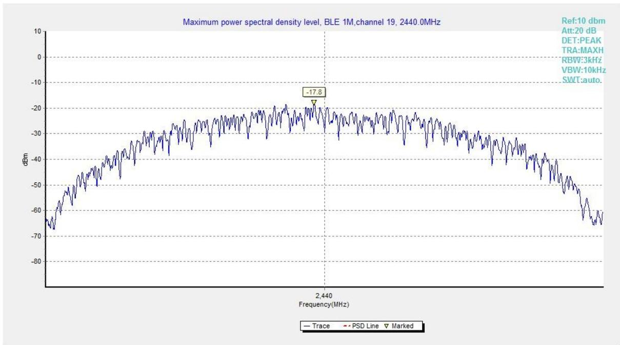
**Fig.2 Power Spectral Density (Ch 19), LE 1M**
