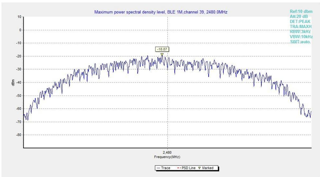
**Fig.3 Power Spectral Density (Ch 39), LE 1M**
