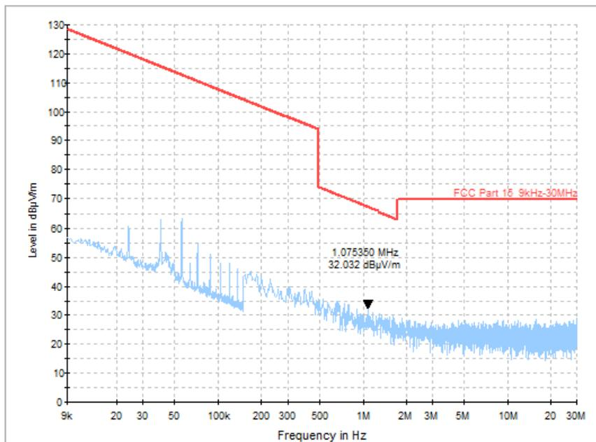
Fig.40 Radiated Spurious Emission (Ch19, 9 kHz - 30 MHz), 1M
