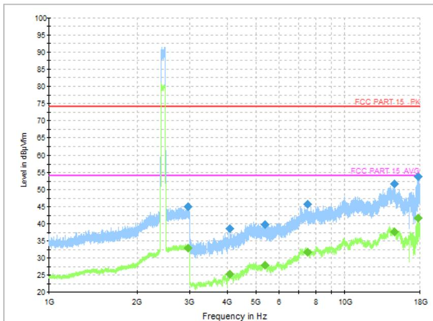
Fig.52 Radiated Spurious Emission (Ch39, 1 GHz - 18 GHz), 2M
