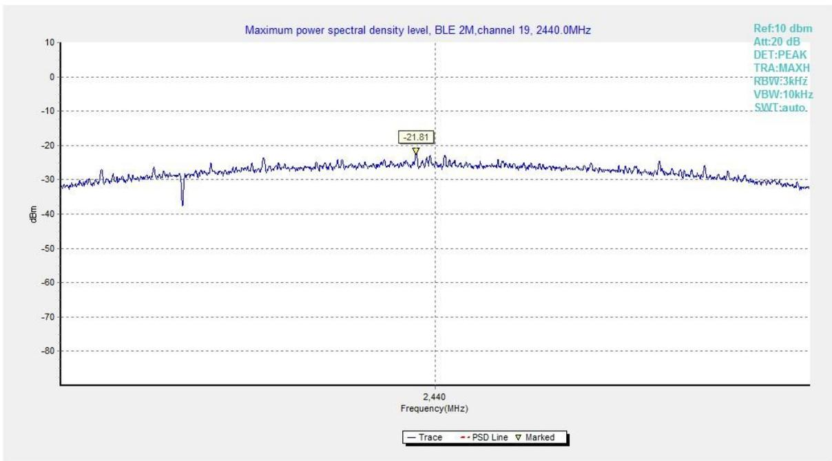
Fig.5 Power Spectral Density (Ch 19), LE 2M
