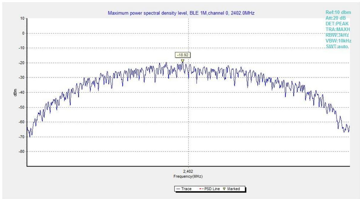
Fig.1 Power Spectral Density (Ch 0), LE 1M
