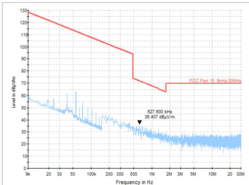
Fig.48 Radiated Spurious Emission (Ch19, 9 kHz - 30 MHz), 2M
