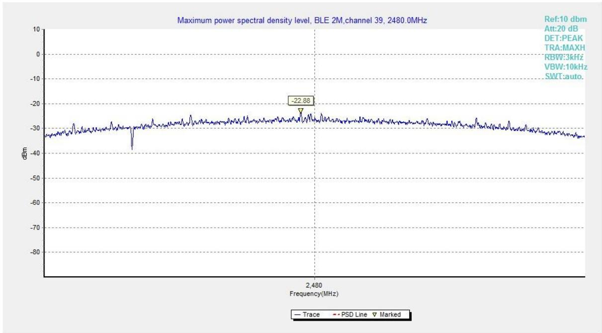
Fig.6 Power Spectral Density (Ch 39), LE 2M
