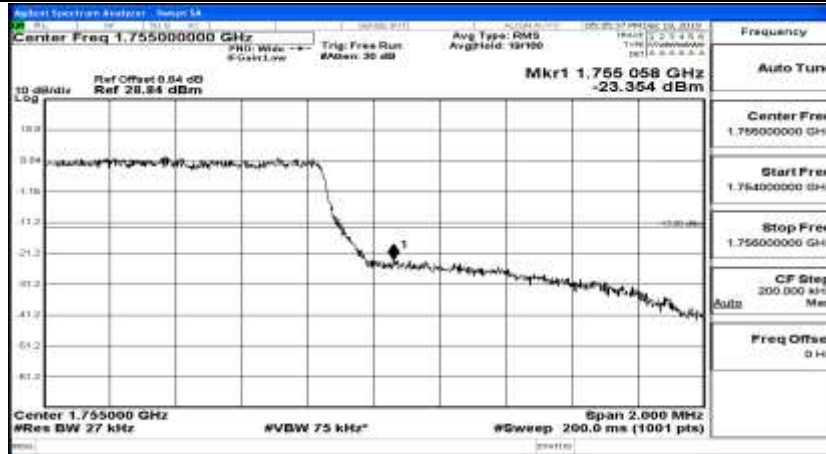
Band Edge Test Graph(s) (Channel Bandwidth: 1.4 MHz)_HCH_16QAM
