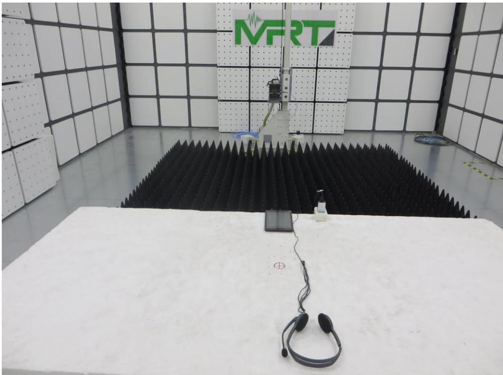
Description: Radiated Emission Test Setup for 30MHz ~ 1GHz (Mode 3)
