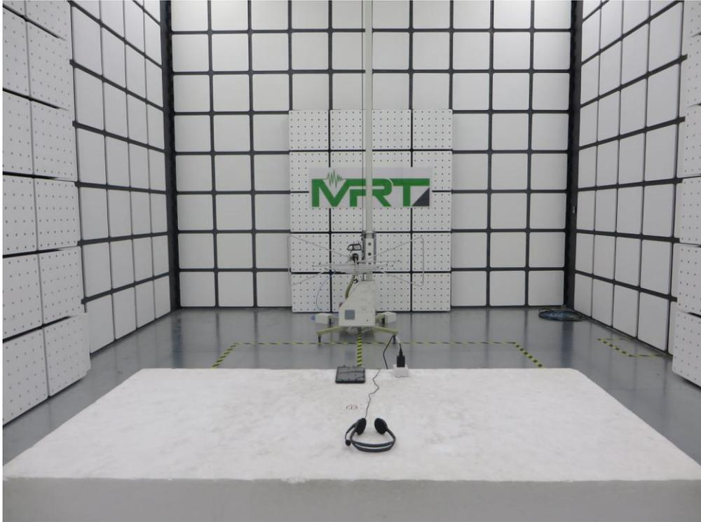
Description: Radiated Emission Test Setup for 1GHz ~ 18GHz (Mode 1 ~ 2)
