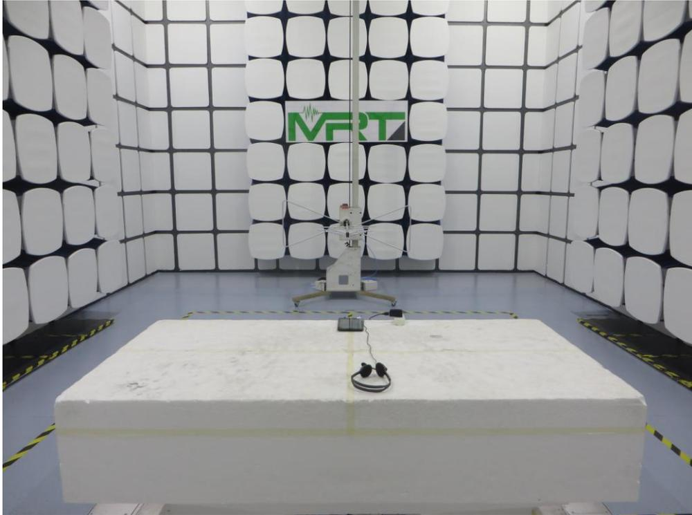
Description: Radiated Emission Test Setup for 1GHz ~ 18GHz (Mode 4)
