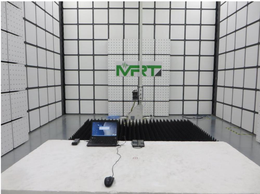
Description: Radiated Emission Test Setup for 30MHz ~ 1GHz (Mode 4)
