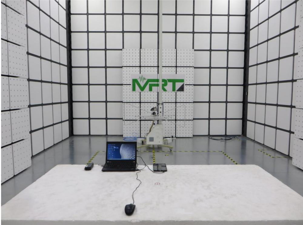
Description: Radiated Emission Test Setup for 1GHz ~ 18GHz (Mode 3)
