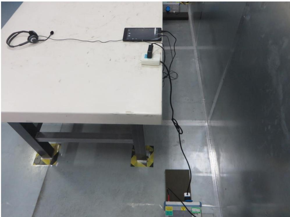
Description: Radiated Emission Test Setup for 30MHz ~ 1GHz (Mode 1 ~ 2)
