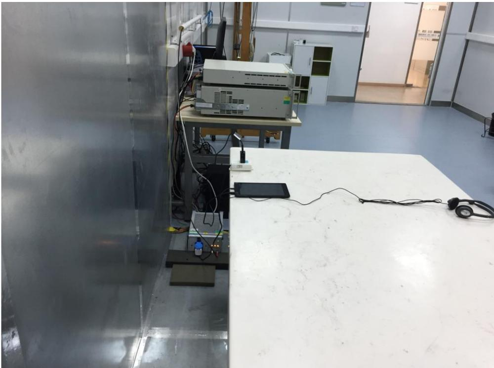
Description: Front view of Conducted Emission Test Setup (Mode 3)
